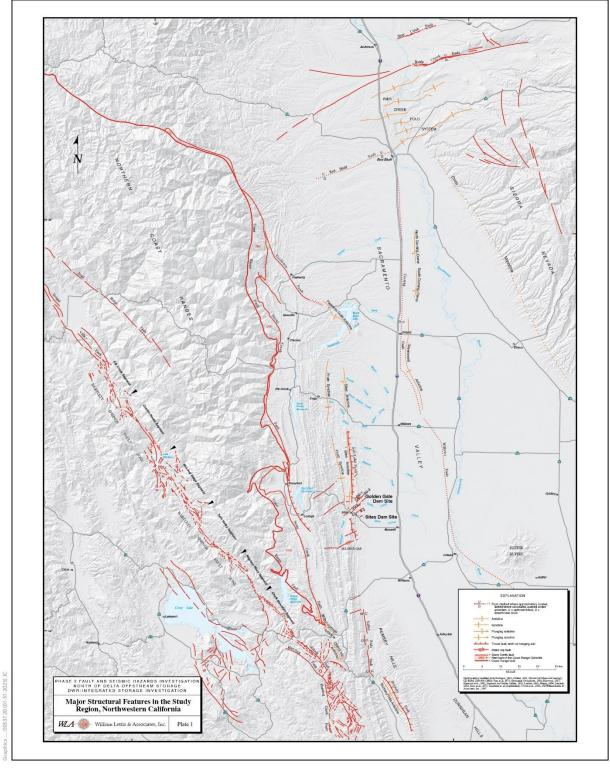
Figure 12-6 Major Structural Features in the Region and the Site-Specific Faults Mapped in the Study Area
