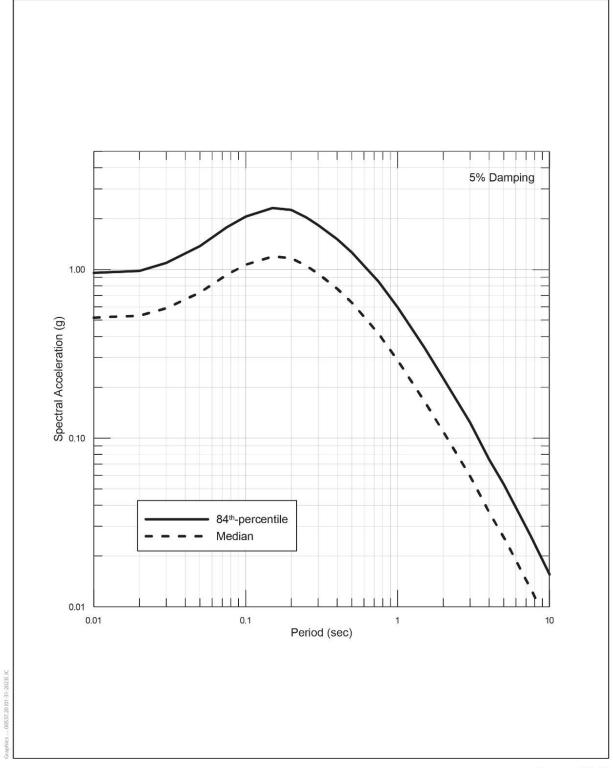
Figure 12-8 Median and 84th Percentile Deterministic Seismic Response Spectra
