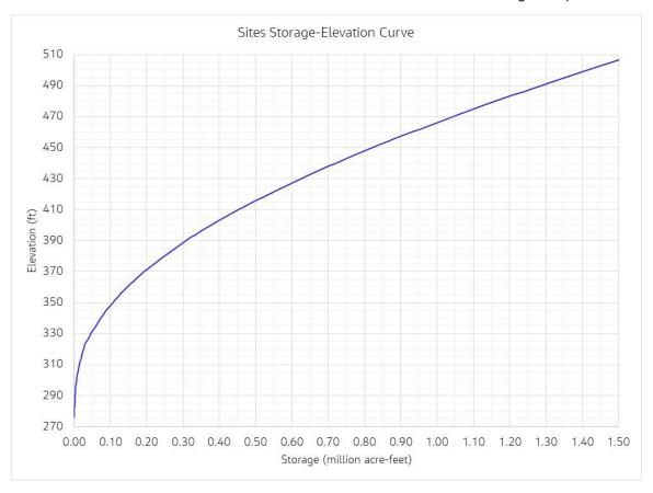
Figure 6D-2. Sites Storage-Elevation Curve
