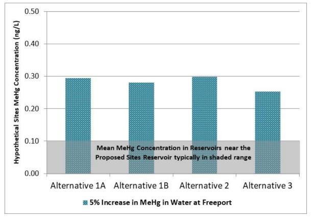
Figure 6F-6. Hypothetical Methylmercury Concentrations in Sites Reservoir Releases Required to Increase Water Column Methylmercury Concentrations in the Sacramento River at Freeport by 5% based on Annual Average Flows.
