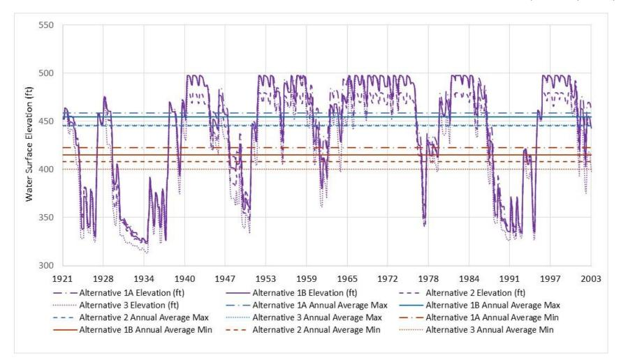
Figure 6F-1. CALSIM Modeled Sites Reservoir Surface Water Elevations and Long-Term Average Annual Maximum and Minimum Surface Water Elevations.
