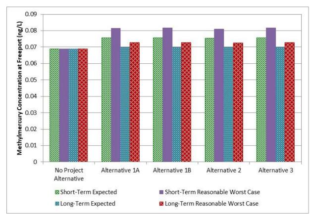
Figure 6F-7. Estimated Surface Water Methylmercury Concentrations at Freeport for Alternatives and the No Project Alternative for Mean Monthly Flows in May – November of Dry and Critical Water Years.
