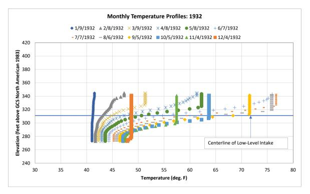
Figure MR4-2. Sites Reservoir Water Temperature Profiles for 1932 Hydrologic Conditions as Simulated with CE-QUAL-W2
