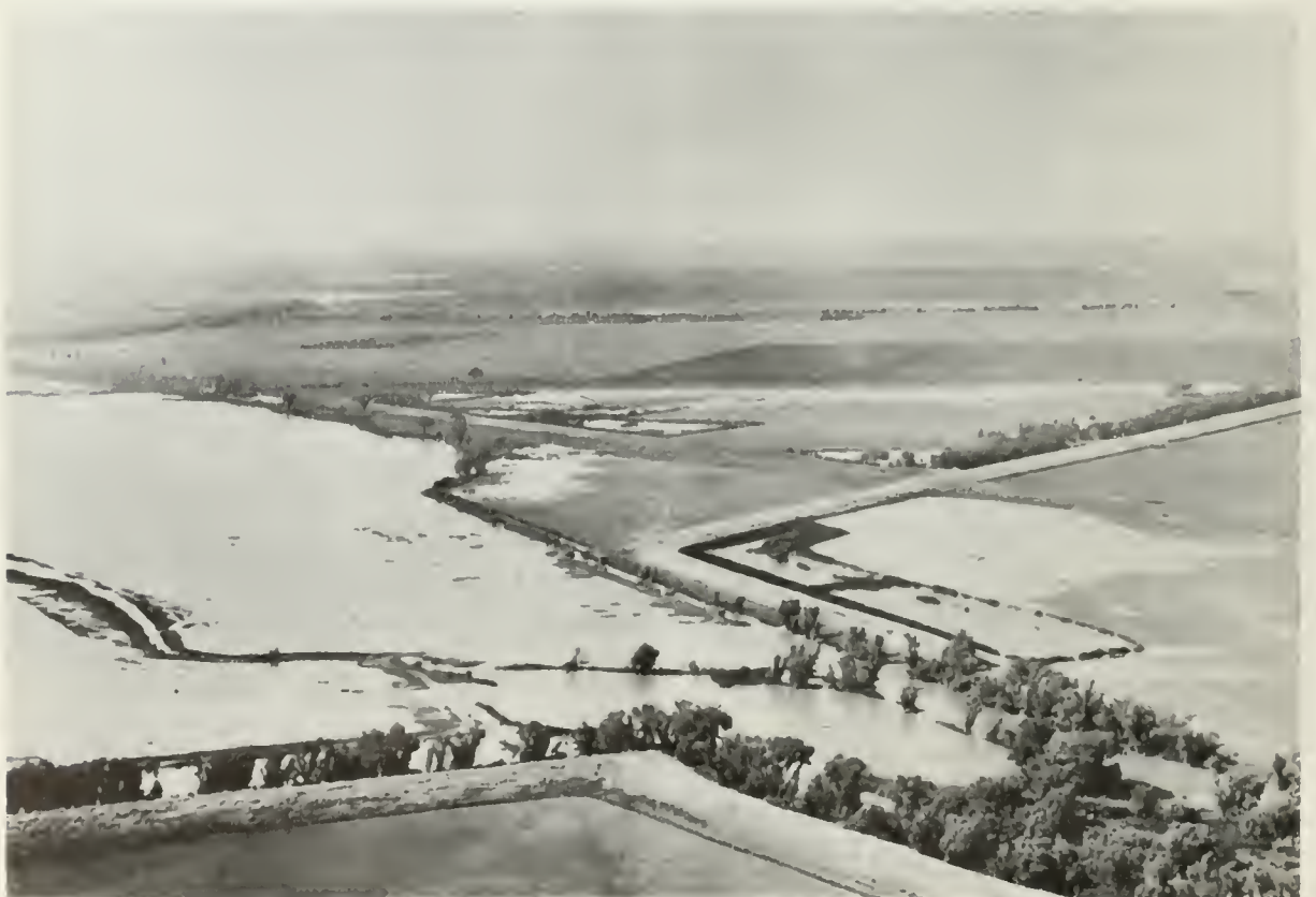
Any flow in excess of 100 second-feet crosses the Yolo Bypass as a sheet.
