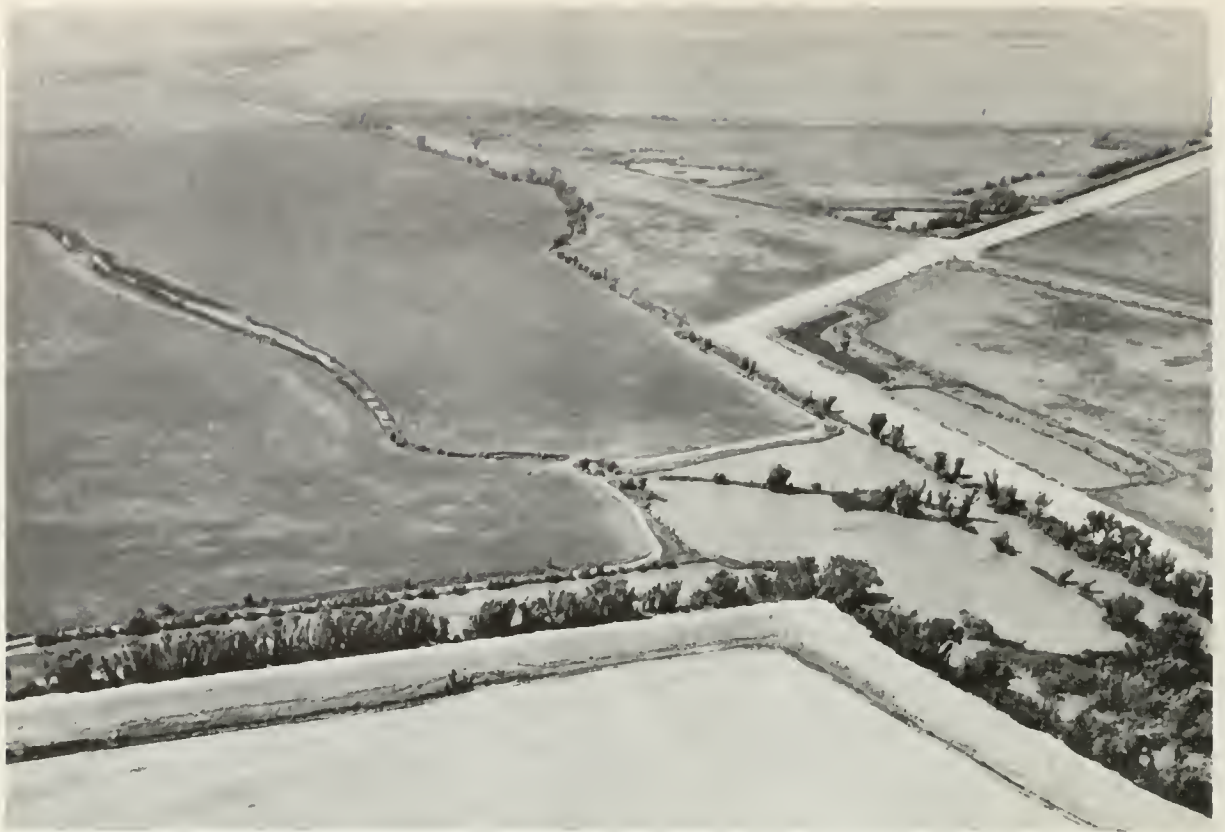
Two small meandering channels constitute the only outlet from the Knights Landing Ridge Cut which is shown above entering the Yolo Bypass from the lower right corner of the photograph.
