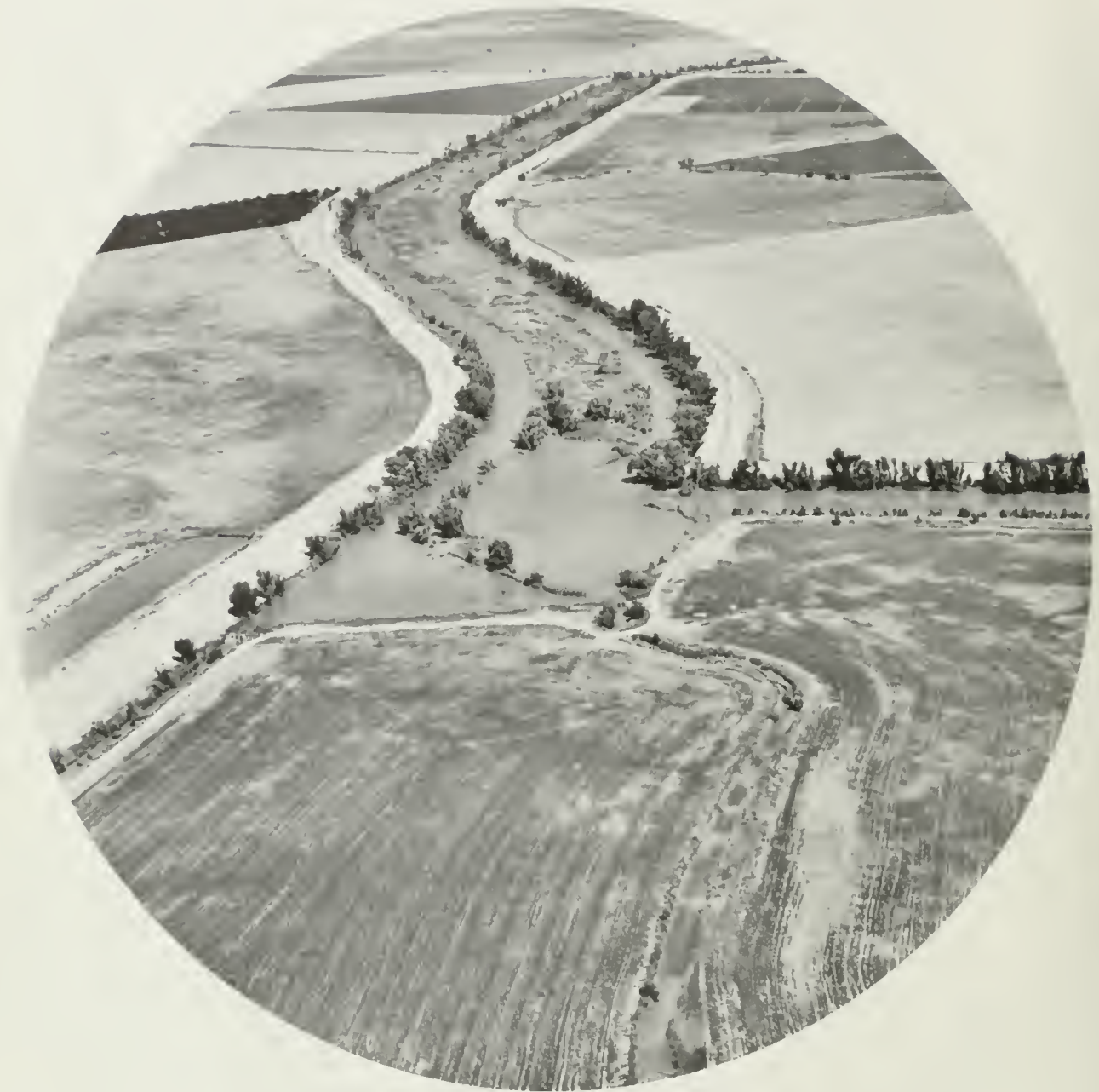
The bottleneck of Colusa Basin drainage where the Knights Landing Ridge Cut meets the Yalo Bypass. Only two small channels (center foreground and at left adjoining road) are available for controlled release of drainage flows.
