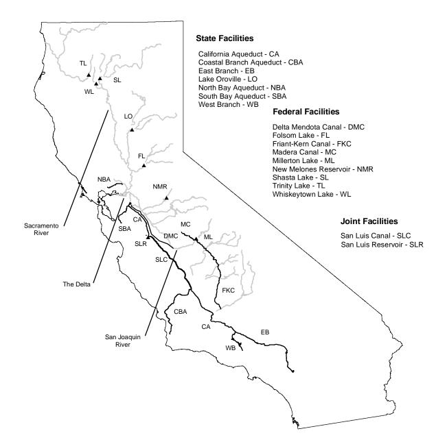
**Fig. 2.** Simplified schematic of CVP-SWP System (CalSim II schematic has considerable greater detail)
