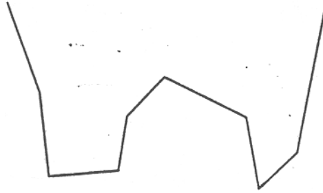
Figure 6.9b “J” Shaped Cross-sections (Should be avoided)
