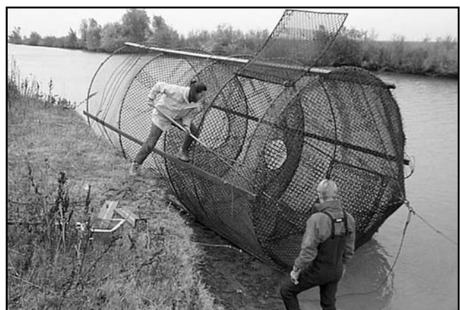
PHOTOGRAPH 1. Fyke trap in operation at the sampling site in the Yolo Bypass Toe Drain.
