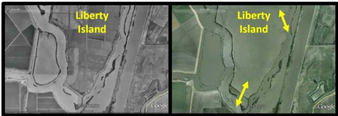
Figure 73. Liberty Island in the north Delta before and after flooding showing locations of narrow breaches in the levee.
