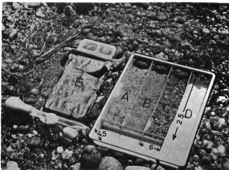
Fig. 49 Experimental trough used to test the burrowing capacity of small ammocoetes. E- holding tray A- mud B- sand C- small gravel D- no cover (measurements in cm.)
