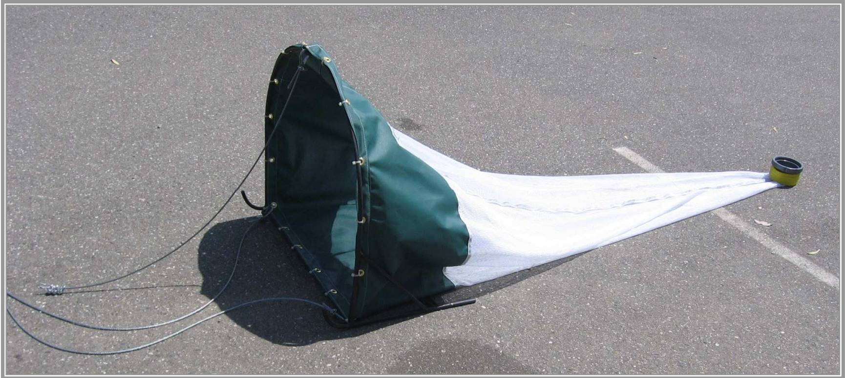
Figure 4. Benthic D-net attached to frame (bucket not attached) used to sample green sturgeon larvae on the upper Sacramento River, CA.
