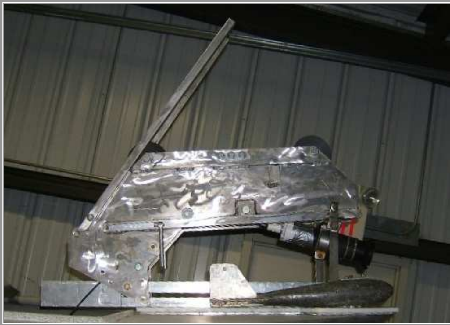
Figure 3. Underwater video camera with sounding weights and carrier positioned in deployment apparatus (Groves and Garcia 1998).
