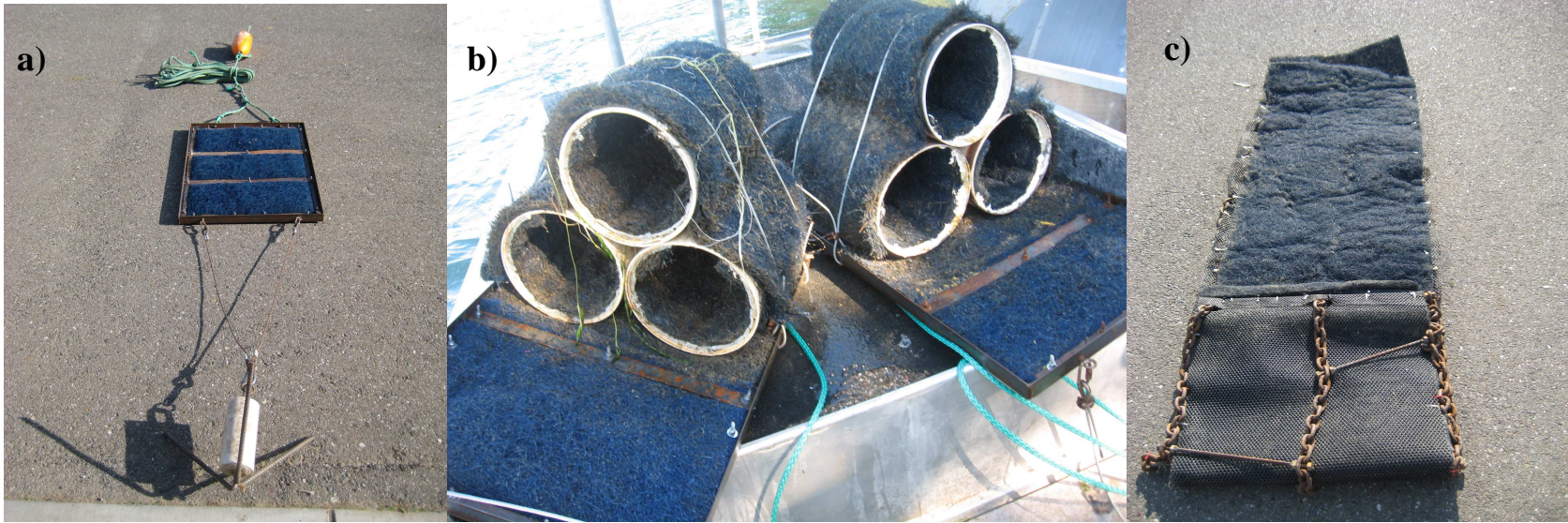
Figure 2. Artificial substrate samplers used to sample for green sturgeon eggs in the upper Sacramento River; a) egg mat; b) egg tube; c) egg roll.
