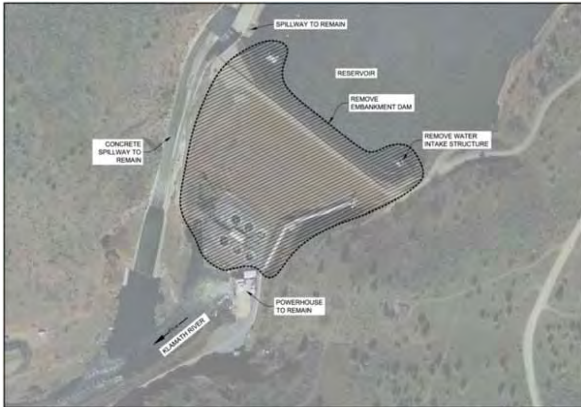
Figure 2-20. Iron Gate dam showing portion of dam to be removed for the Partial Facilities Removal Alternative.
