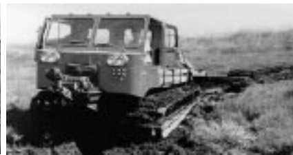
DMC 1200 scavel ditching
