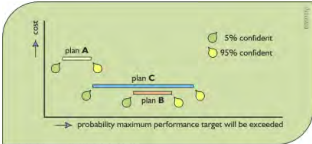
Figure 23. Tradeoffs among cost, reliabilities, and the confidence level of those reliabilities. The relative ranking of plans with respect to the probability of exceeding the desired (maximum limit) target may depend on the confidence given to that probability.
