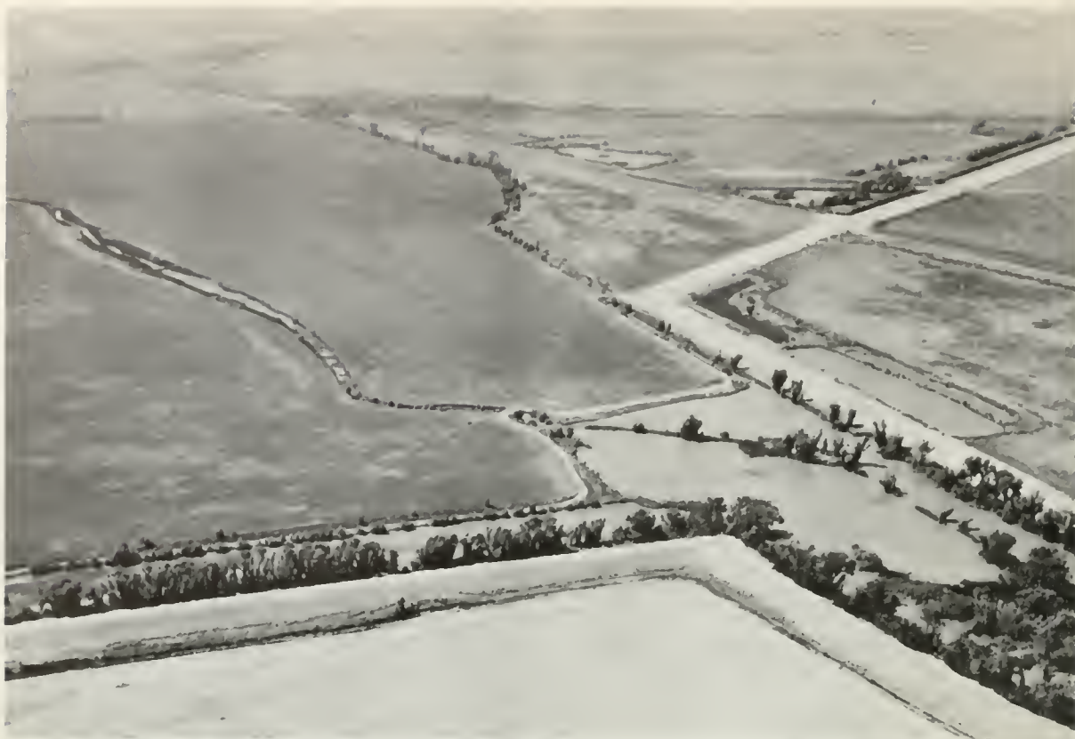
Two small meandering channels constitute the only outlet from the Knights Landing Ridge Cuf which is shown above entering the Yolo Bypass from the lower right corner of the photograph.
