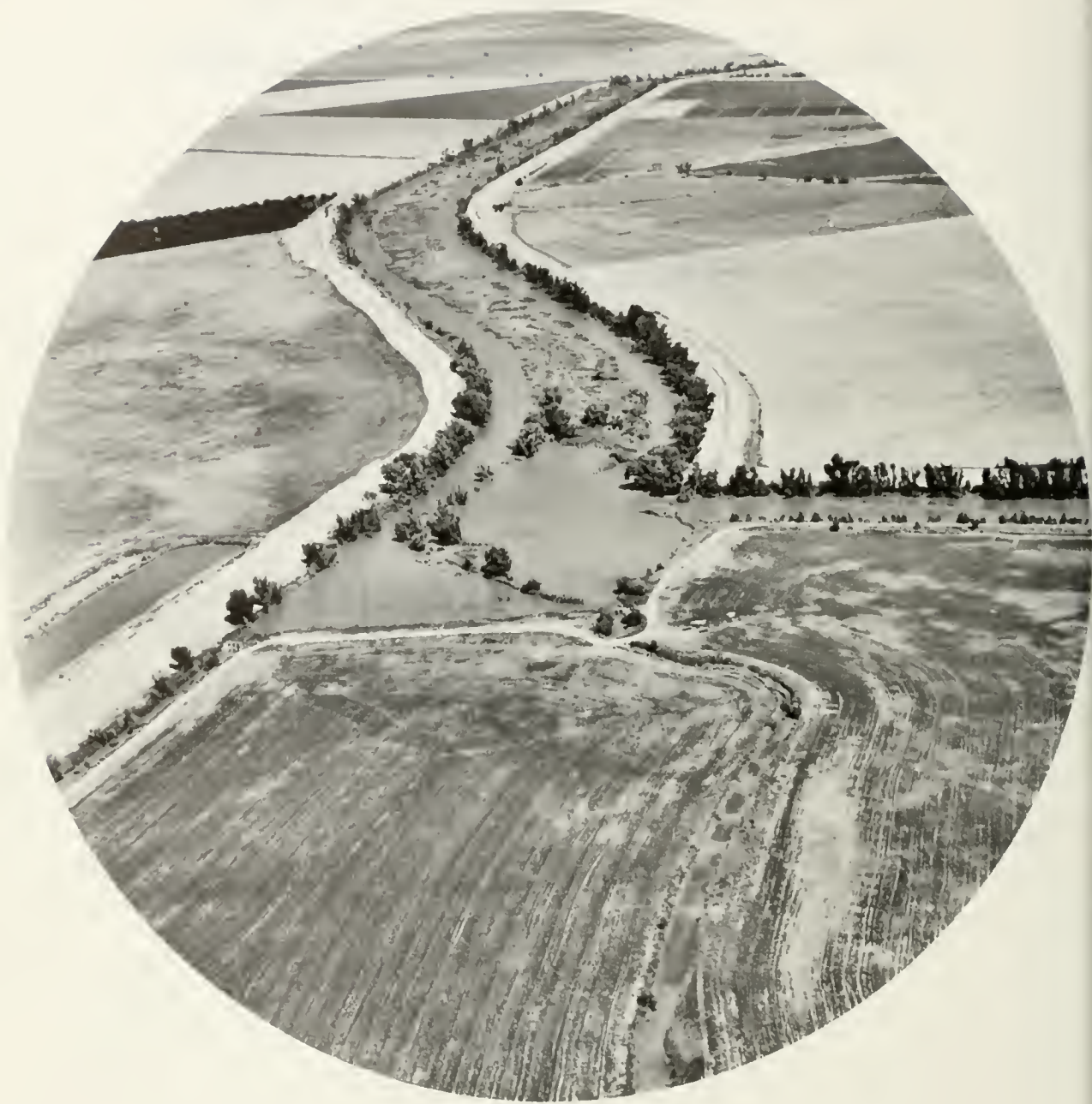
The bottleneck of Colusa Basin drainage where the Knights Landing Ridge Cut meets the Yolo Bypass. Only two small channels (center foreground and at left adjoining road) are available for controlled release of drainage flows.
