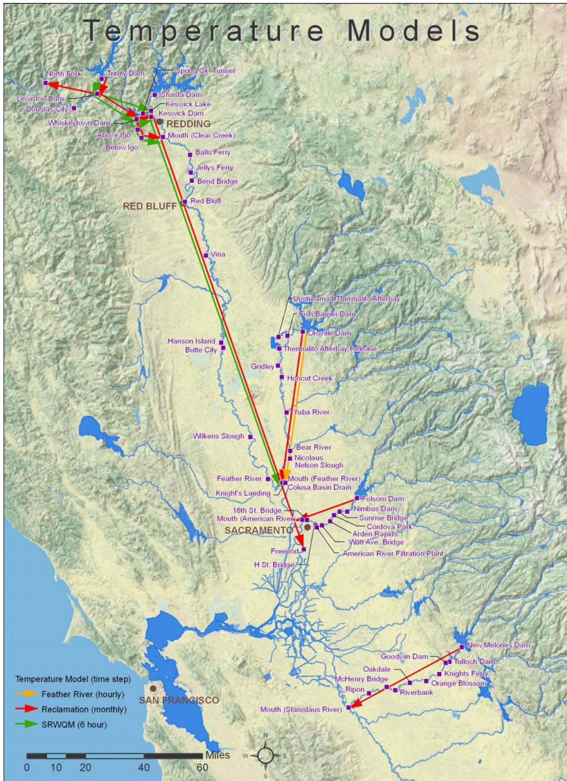
Figure 9-5 General spatial representation of the temperature model networks.
