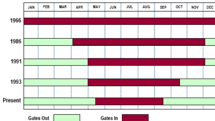
Figure 8-14. Historical patterns of gate operations at Red Bluff Diversion Dam.
