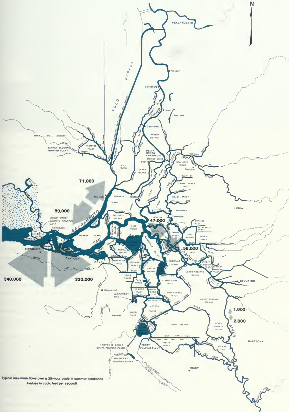
Figure 10-3. Tidal Flows in the Sacramento-San Joaquin Delta (in cubic feet per second)
