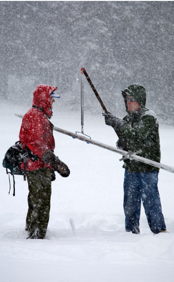
Snow surveyors measure the water content of the Sierra snowpack, to forecast water supply conditions for the upcoming dry season.
