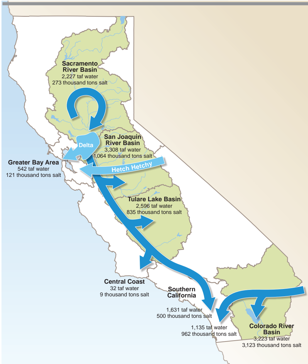
Figure 19-4 Movement of Salts in California from the Major Federal and State Water Projects
