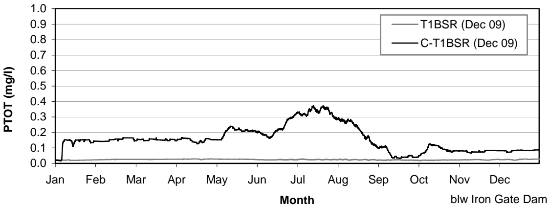
Figure C11: Total phosphorus below Iron Gate dam under Revised Draft TMDL “natural” baseline scenario (T1BSR) and under the modified “natural” baseline scenario (C-T1BSR)
