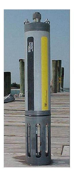
This is a YSI 6000 UPG Multi-Parameter Water Quality Monitor. This particular model measures dissolved oxygen, salinity, temperature, pH, depth, and turbidity. Click on image for more details. (Photo: North Carolina NERRS site)
