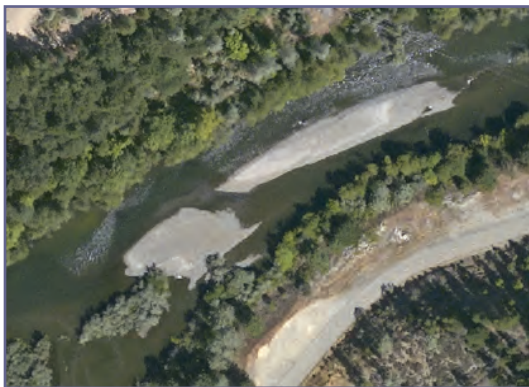
Bear Island near Lewiston. The bar is growing in response to upstream gravel augmentation and high flow releases.
