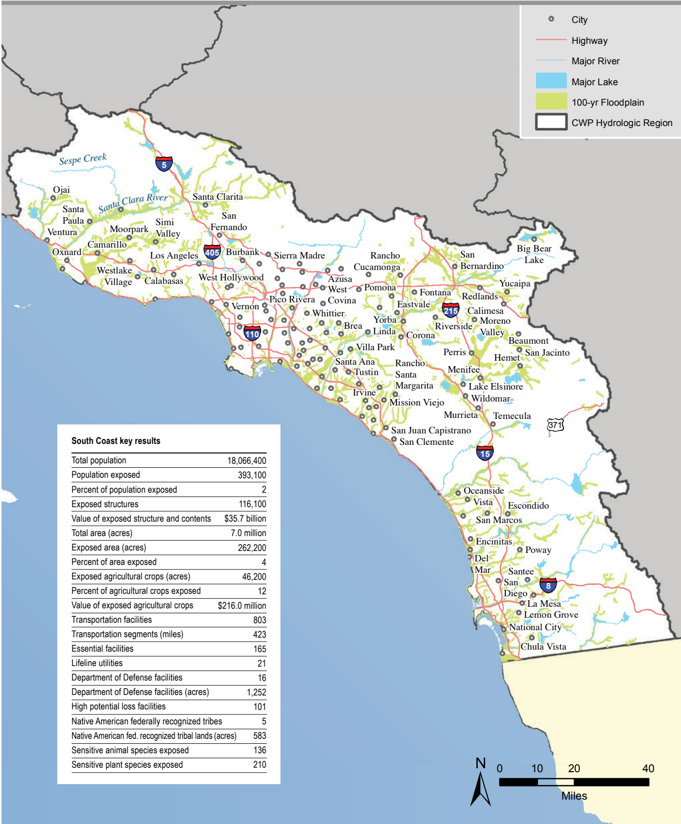
Figure SC-16 Flood Hazard Exposure to the 100-Year Floodplain in the South Coast Hydrologic Region
