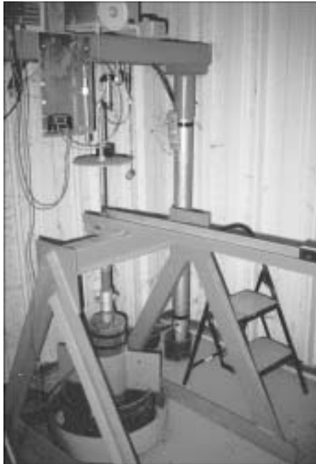
Figure 19 Photograph of extensometer
