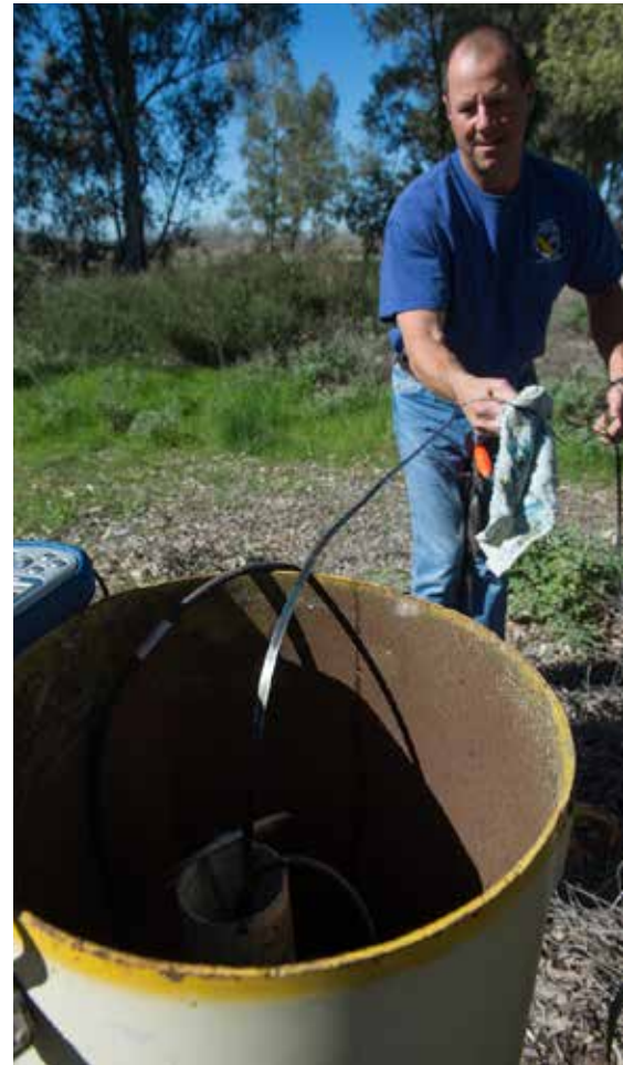
DWR staff measuring the groundwater level in a monitoring well
