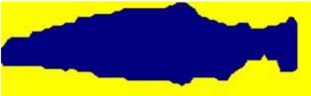
Figure 6. Infrared silhouettes created from the O. mykiss as it passed through the Vaki scanner and into the trap. These silhouettes are very similar to the Chinook silhouettes and without a digital photograph could have easily been mistaken for a Chinook. Images obtained from Stanislaus weir e-mail summary (2005).
