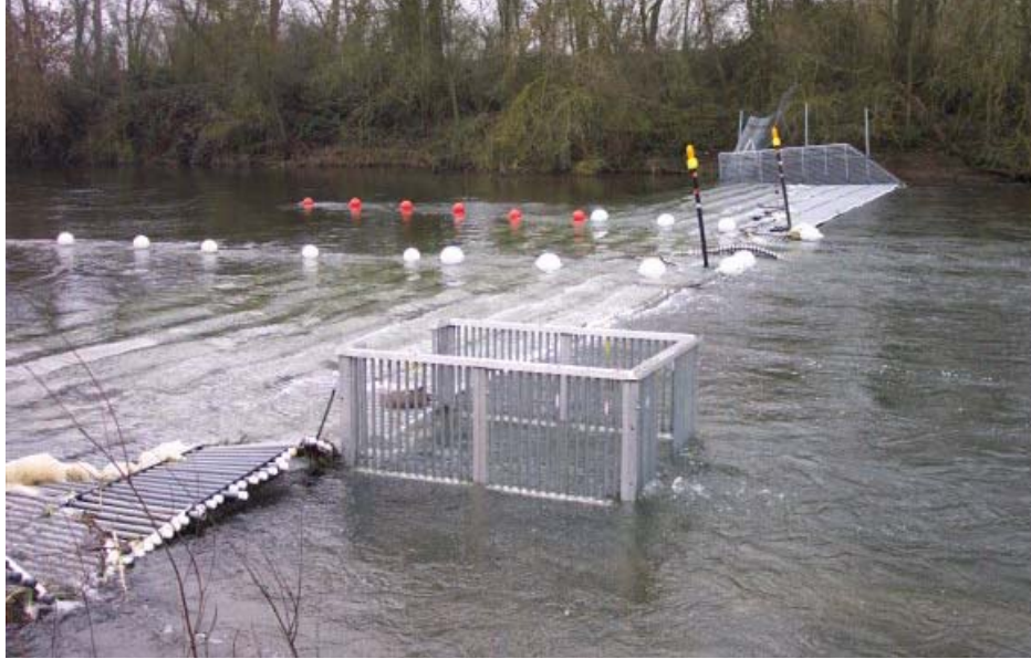
Figure 4. Resistance board weir (Alaskan style) with a Vaki Riverwatcher System on the Stanislaus River, CA. Photo credit: David Hu, USFWS.
