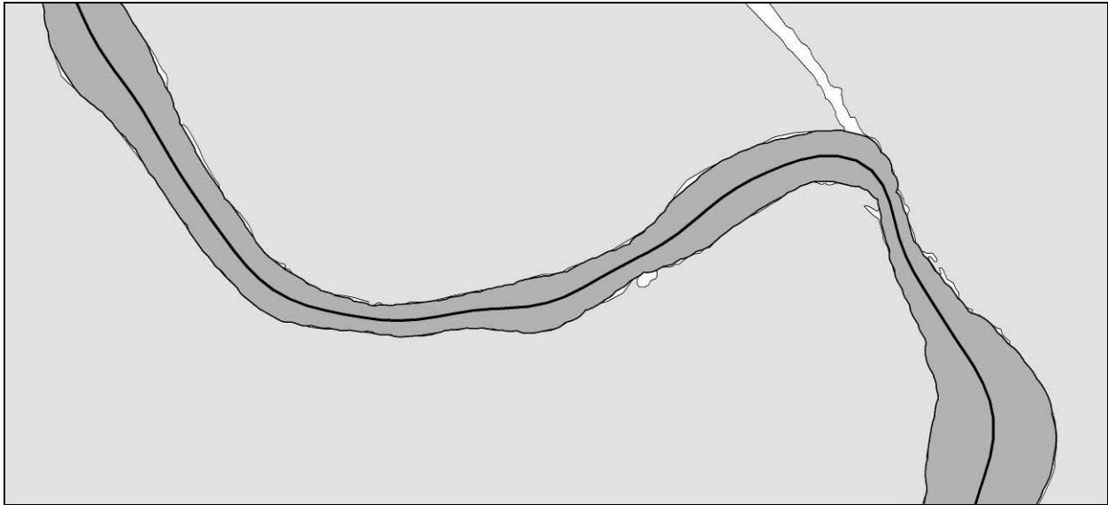
Figure 4.5. Simplified channel for initial conditions.
