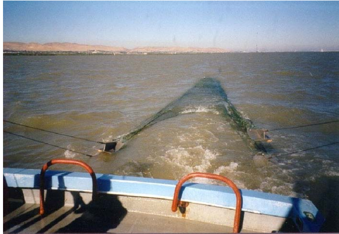
Photo 9 Chipps Island Trawl: The Chipps Island trawl off the stern of the Research Vessel Whitesel during net retrieval.
