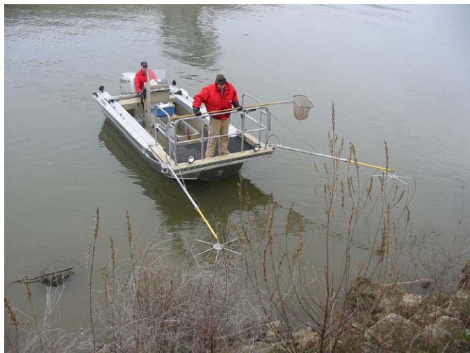
Photo 7 Resident Fishes Survey. Fish within a created electrical field are attracted to boat's forward-mounted anode probes.
