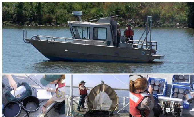
Photo 5 20 mm Survey. Clockwise from top, Research Vessel Munson tows 20 mm net; ichthyo-samples prior to return to the lab; mouth view of 20 mm net with zooplankton net on top; measuring water temperature and electrical conductivity.
