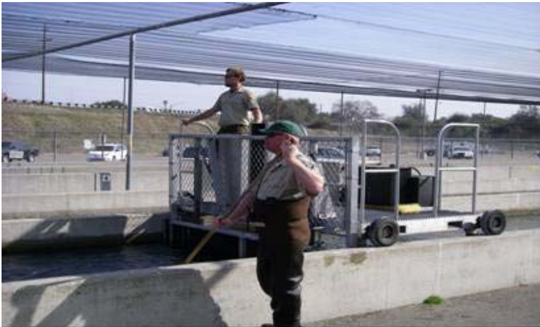
Figure 4-22. Gasoline operated mechanical fish crowder in the raceway.
