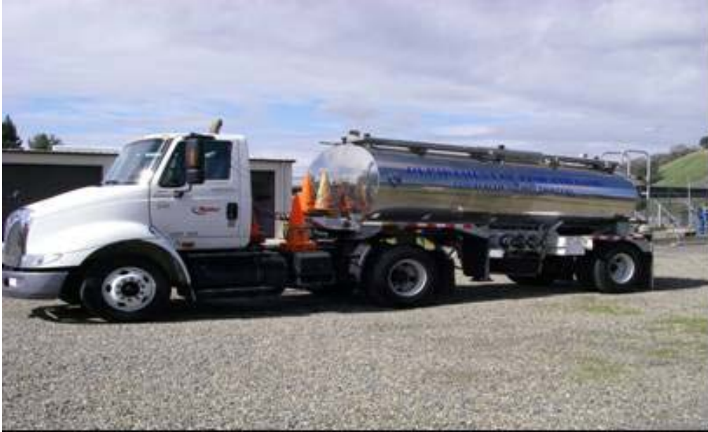
Figure 4-24. 2,800-gallon West-Mark ST-2800 NS fish hauling tank with tractor.
