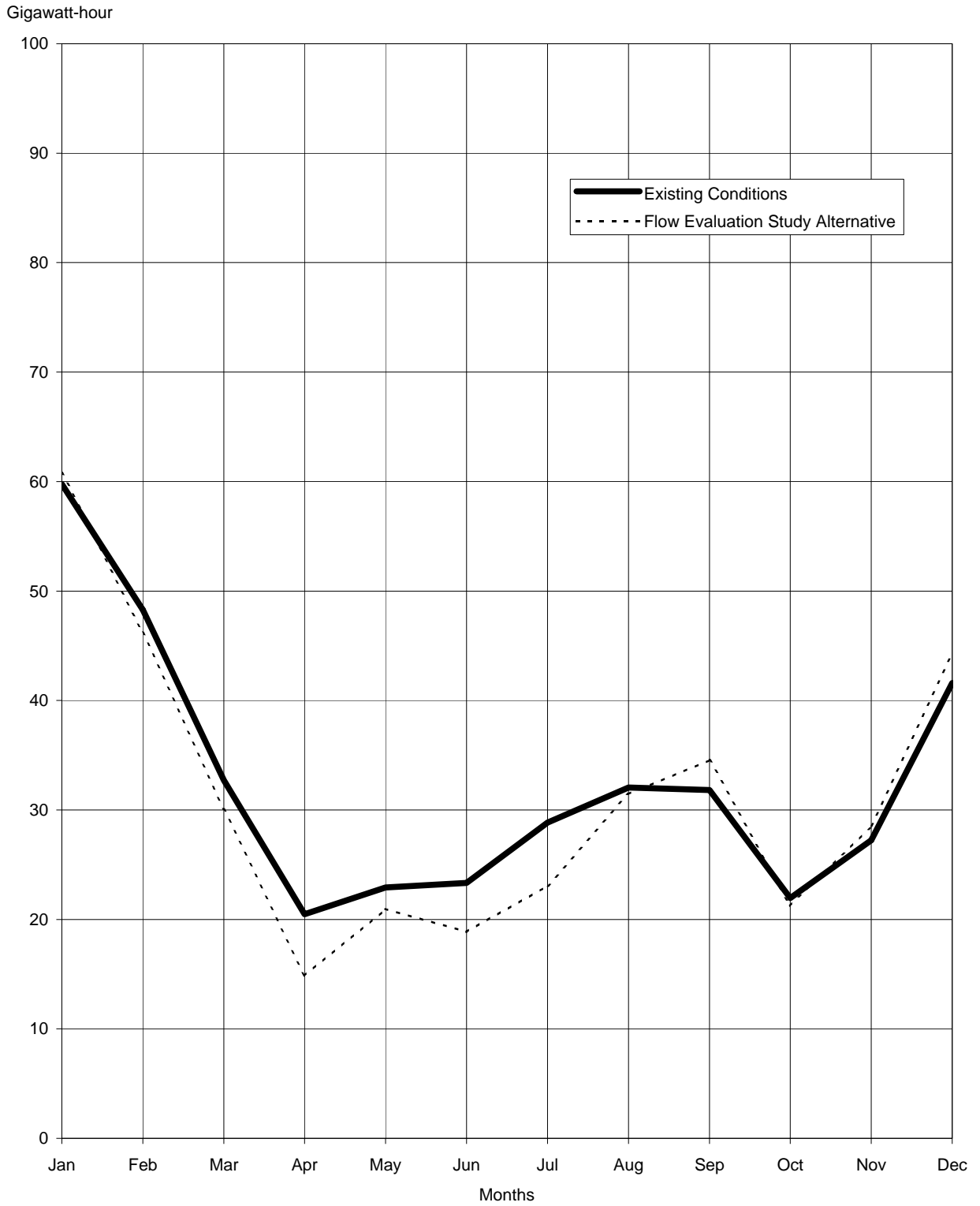
FIGURE F-27 SIMULATED AVERAGE MONTHLY ON-PEAK CVP PROJECT USE ENERGY DRY PERIOD 1928-1934
