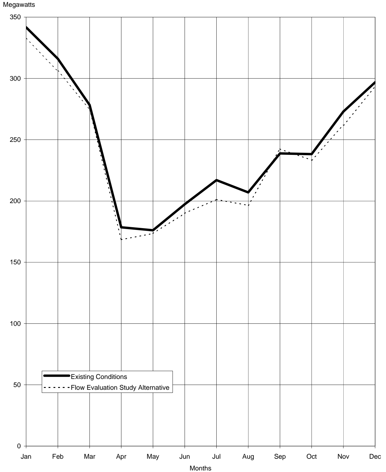
FIGURE F-30 SIMULATED AVERAGE MONTHLY OFF-PEAK CVP PROJECT USE CAPACITY LONG-TERM AVERAGE 1922-1990
