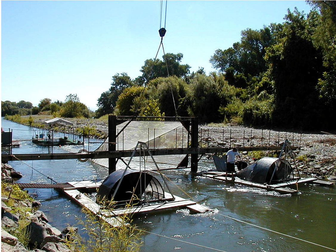
Figure 4. Fyke net and two rotary screw traps used to recapture test, control, and weir groups of marked fish during the 2003 and 2004 biological evaluations at GCID. Prior to release of fish, the 60-ft. long fyke net was lowered in the channel current by crane into the H-pile slots. Recaptured fish were accumulated in the floating live box attached to the end of the fyke net and rotary screw trap live boxes, and then examined for marks to identify initial release location.
