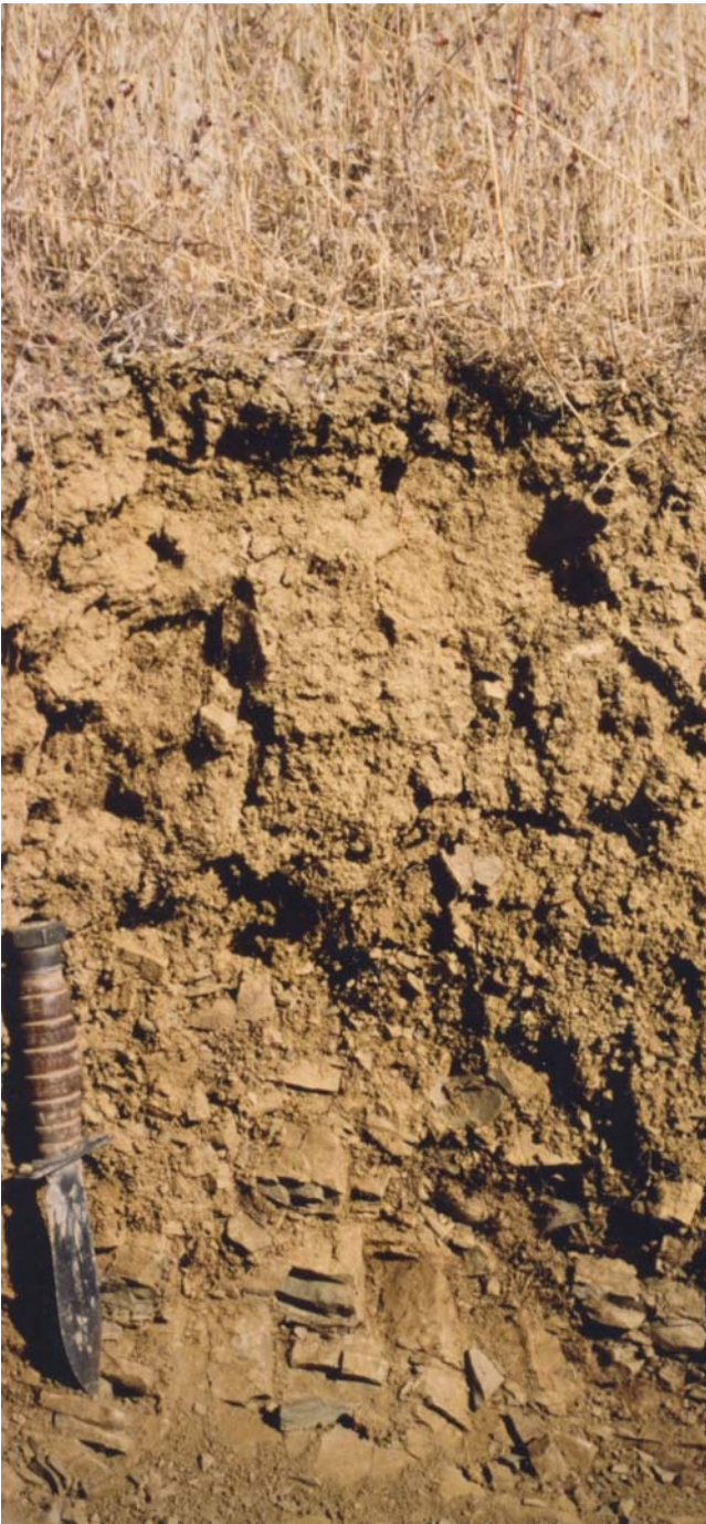
Figure 19.—Profile of Millsholm soils, which are shallow over sandstone. The knife is 8 inches long.
