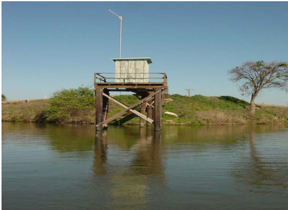
Photograph 5.3-2. Water Quality Monitoring Station on Old River at the Head of Middle River (on right) This tidal stage and salinity (EC) measurement station is called Union Island by the Bureau of Reclamation (Source: California Department of Water Resources.)
