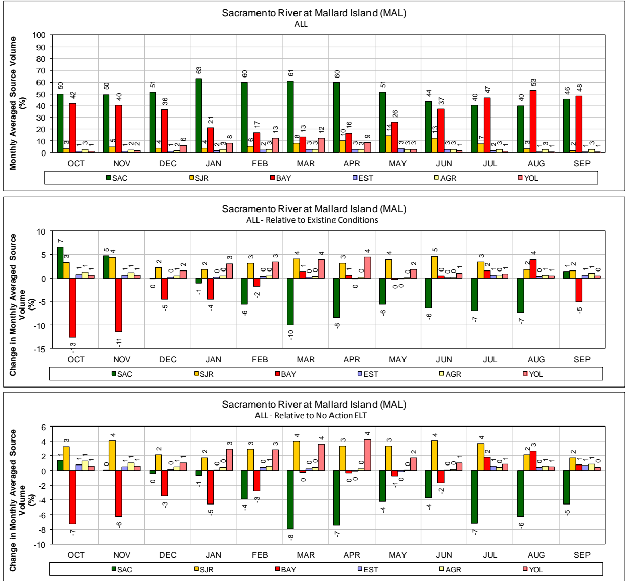
1 2 Figure B.4-57. ALT 4A Scenario H4 – Sacramento River at Mallard Island for ALL Years (1976–1991) 3 Monthly average source volume (top figure) and change in monthly average source volume relative to 4 Existing Conditions and No Action Alternative Early Long Term (bottom two figures). 5
