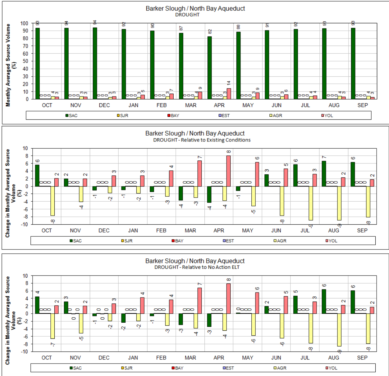
1 2 Figure B.4-82. ALT 2D – North Bay Aqueduct at Barker Slough Pumping Plant for DROUGHT Years 3 (1987–1991)
