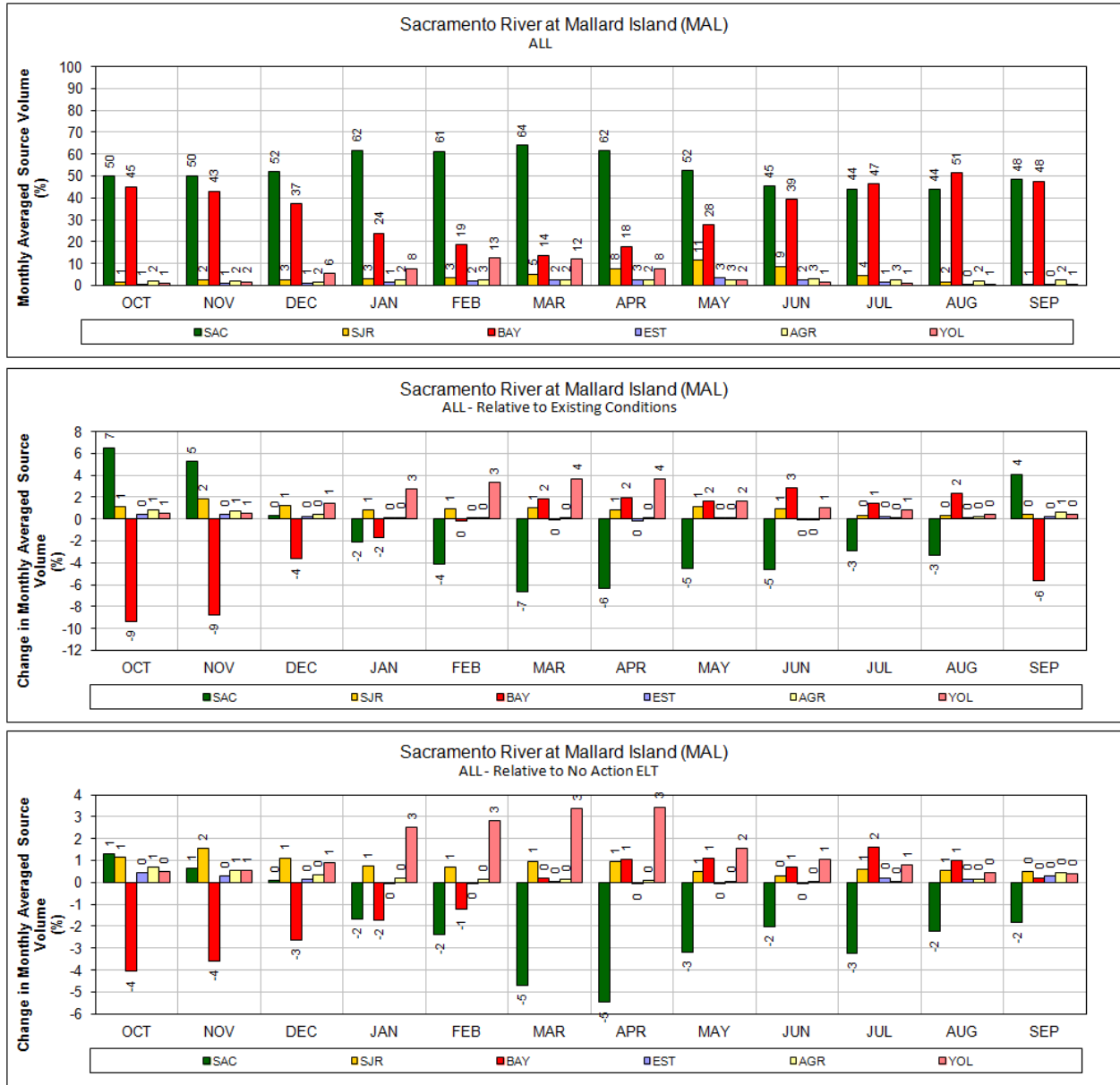
1 2 Figure B.4-101. ALT 5A – Sacramento River at Mallard Island for ALL Years (1976–1991) 3 Monthly average source volume (top figure) and change in monthly average source volume relative to 4 Existing Conditions and No Action Alternative Early Long Term (bottom two figures). 5
