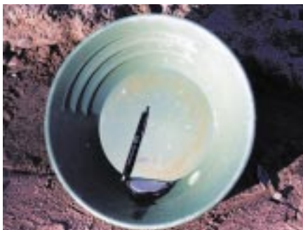
Figure 2. Gold pan with more than 30 grams of mercury from 1 kilogram of mercury-contaminated sediments.
