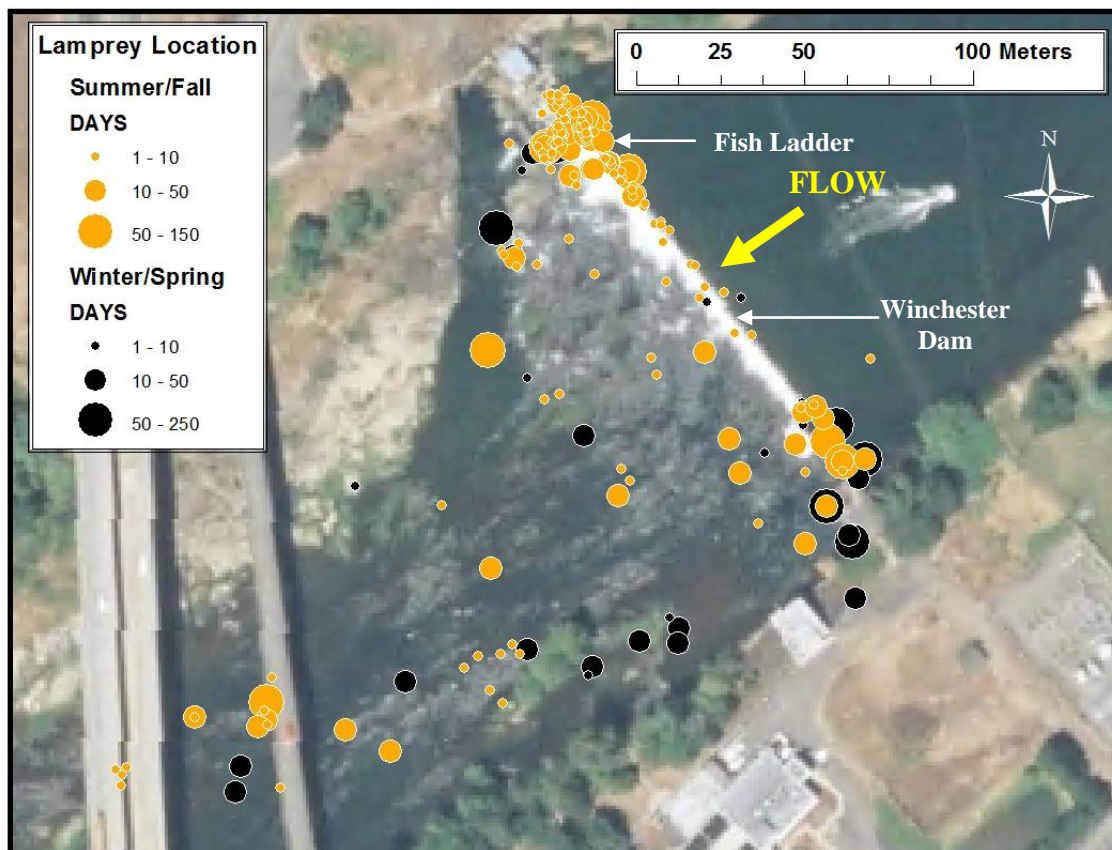
Figure 3.4. Locations of the tagged lamprey at Winchester Dam during the summer/fall season (2009 and 2010 data) and winter/spring season (2009 data). Each circle represents a specific detection location of a tagged lamprey and the number of days spent at each location is represented by the size of the circle.
