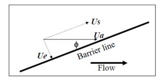
Note: *Ua* is the channel velocity, *Ue* is the fish escape velocity, and *Us* is the sweeping velocity component along the face of the barrier (Turnpenny and O'Keeffe 2005).
