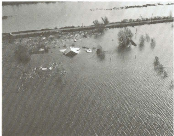
A combination of high tides, winter floodflows, and poor levees can result in flooded islands.
