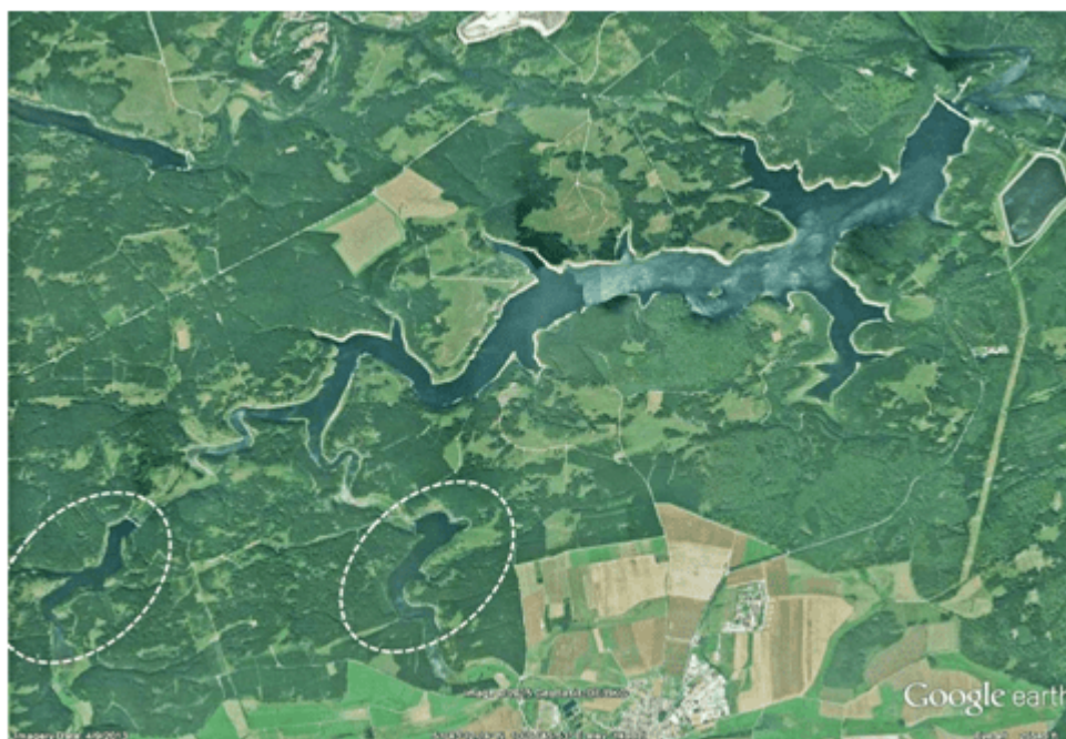
Figure 4.5. Rappbode Reservoir, Germany with two pre-dams (lower left corner). Photo credit: Google Earth.
