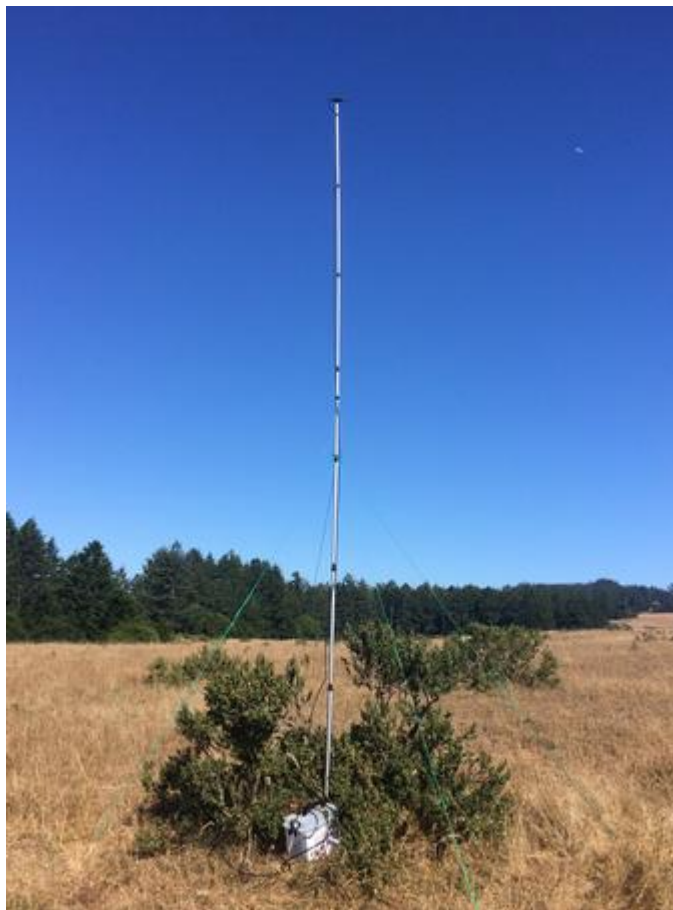
This device collects vocalization emitted by bats. Scientists use the recordings from these devices to determine what species are using the area. (Credit: Gabe Reyes, USGS, WERC. Public domain.)
