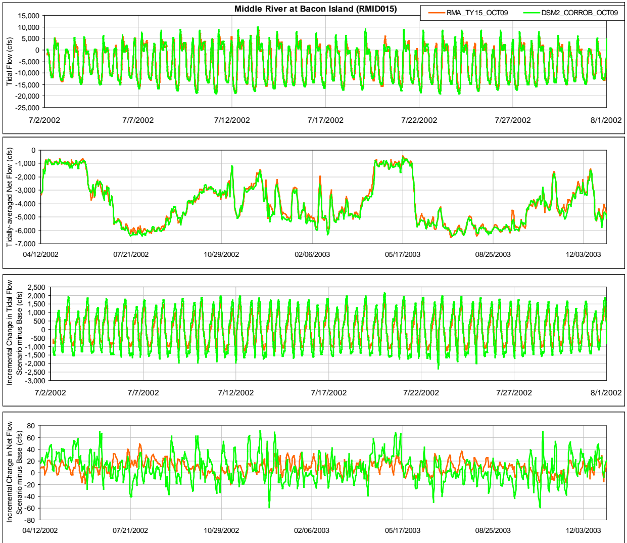
1 Figure 1-54. Comparison of Tidal Flow, Tidally-Averaged Daily Flow, Incremental Change in Tidal 2 Flow and the Incremental Change in the Daily Flow between the Early Long-term Scenario and the 3 Current Conditions Scenario from RMA Model and DSM2 Model for Middle River at Bacon Island 4 Location
