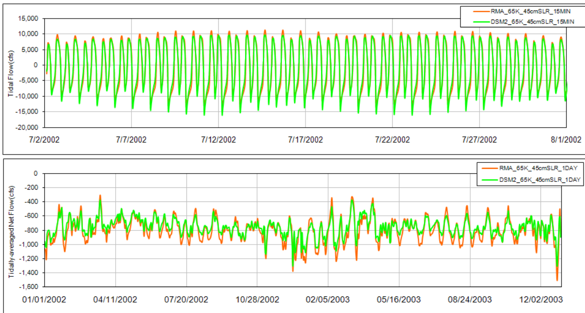
6 Figure 1-203. Comparison of Tidal Flow and Tidally-Averaged Daily Flow between the Integrated Late 7 Long-term Scenario and the Current Conditions Scenario from RMA Model and DSM2 Model for Suisun 8 Island 10 Breach 3 under Suisun Marsh Region.
