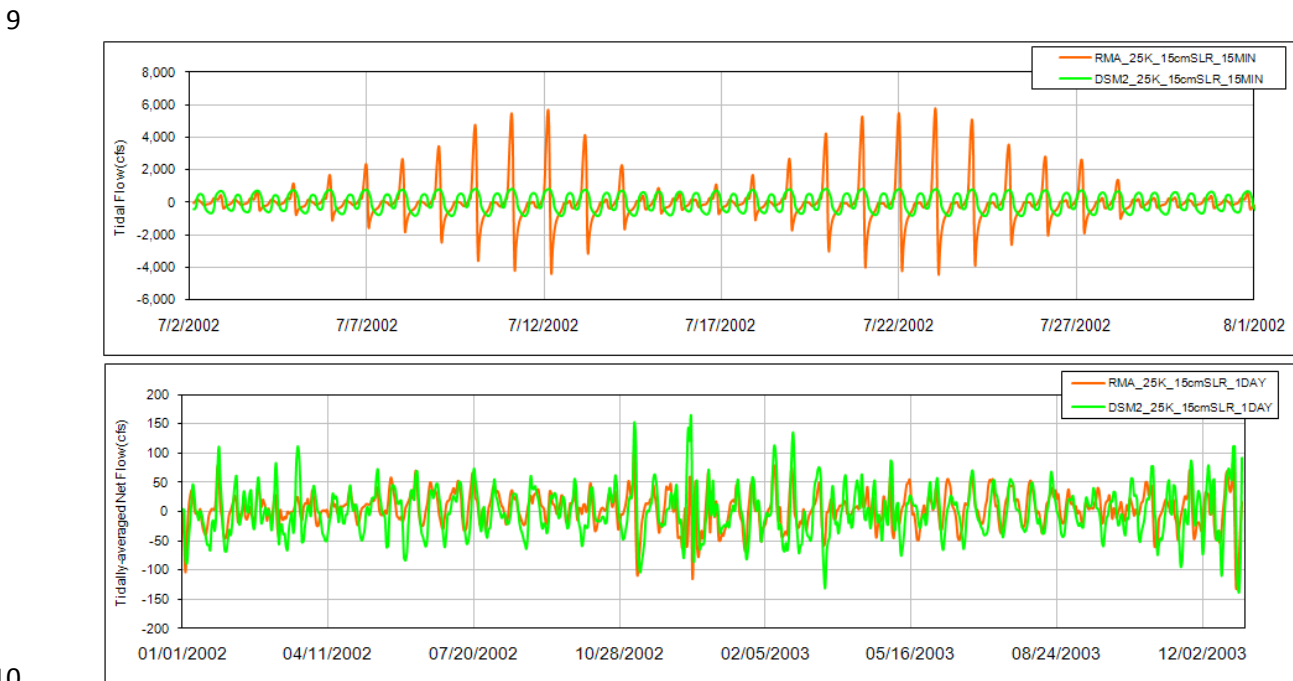
5 6 Figure 1-164. Comparison of Tidal Flow and Tidally-Averaged Daily Flow between the Integrated Early 7 Long-term Scenario and the Current Conditions Scenario from RMA Model and DSM2 Model for 8 Montezuma Wetlands North and South breaches under Cache Region.
