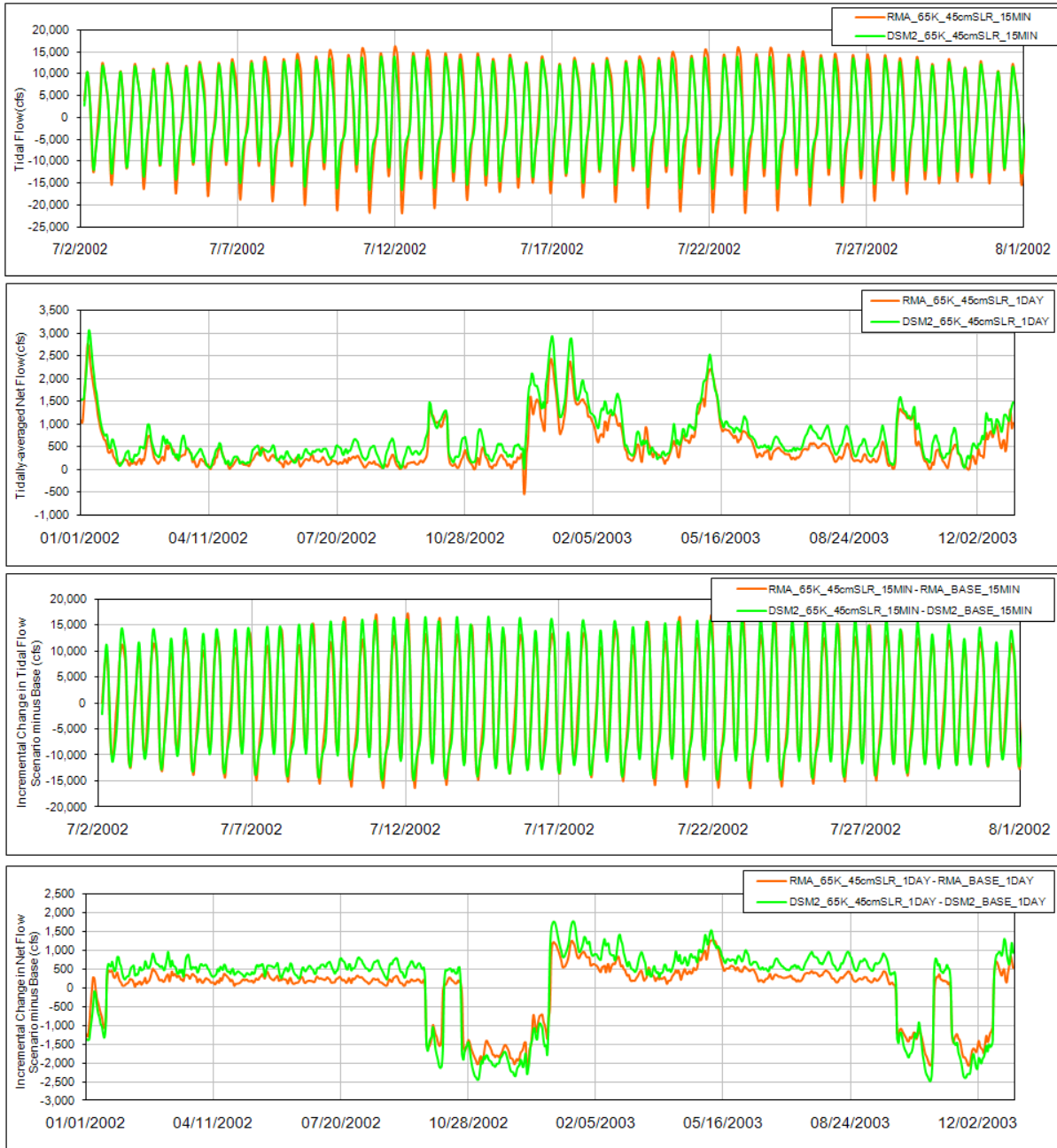
1 Figure 1-192. Comparison of Tidal Flow, Tidally-Averaged Daily Flow, Incremental Change in Tidal Flow 2 and the Incremental Change in the Daily Flow between the Integrated Late Long-term Scenario and the 3 Current Conditions Scenario from RMA Model and DSM2 Model for Montezuma Slough at Head Location. 4
