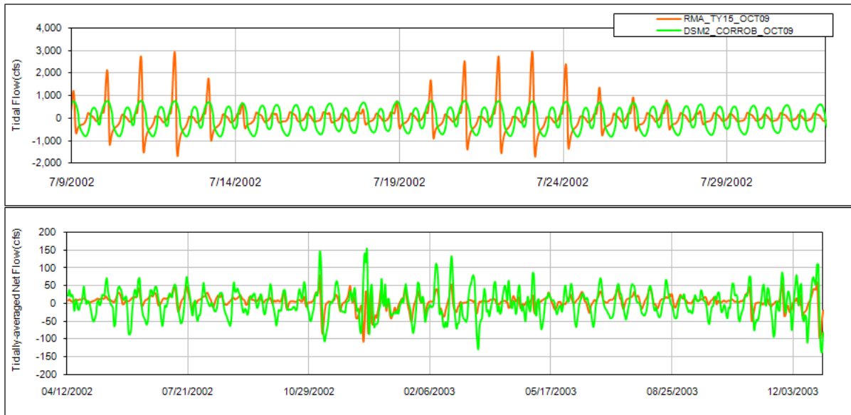
7 Figure 1-96. Comparison of Tidal Flow and Tidally-Averaged Daily Flow between the Late Long-Term 8 Scenario and the Current Conditions Scenario from RMA Model and DSM2 Model for Montezuma 9 Wetlands Breach under Suisun Marsh
