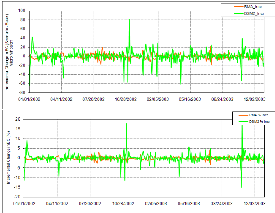
4 5 Figure 1-187. Comparison of Tidally-Averaged Daily EC and the Incremental Change in the Daily EC 6 between the Integrated Early Long-Term Scenario and the Current Conditions Scenario from RMA Model 7 and DSM2 Model for Middle River at Middle River Location.
