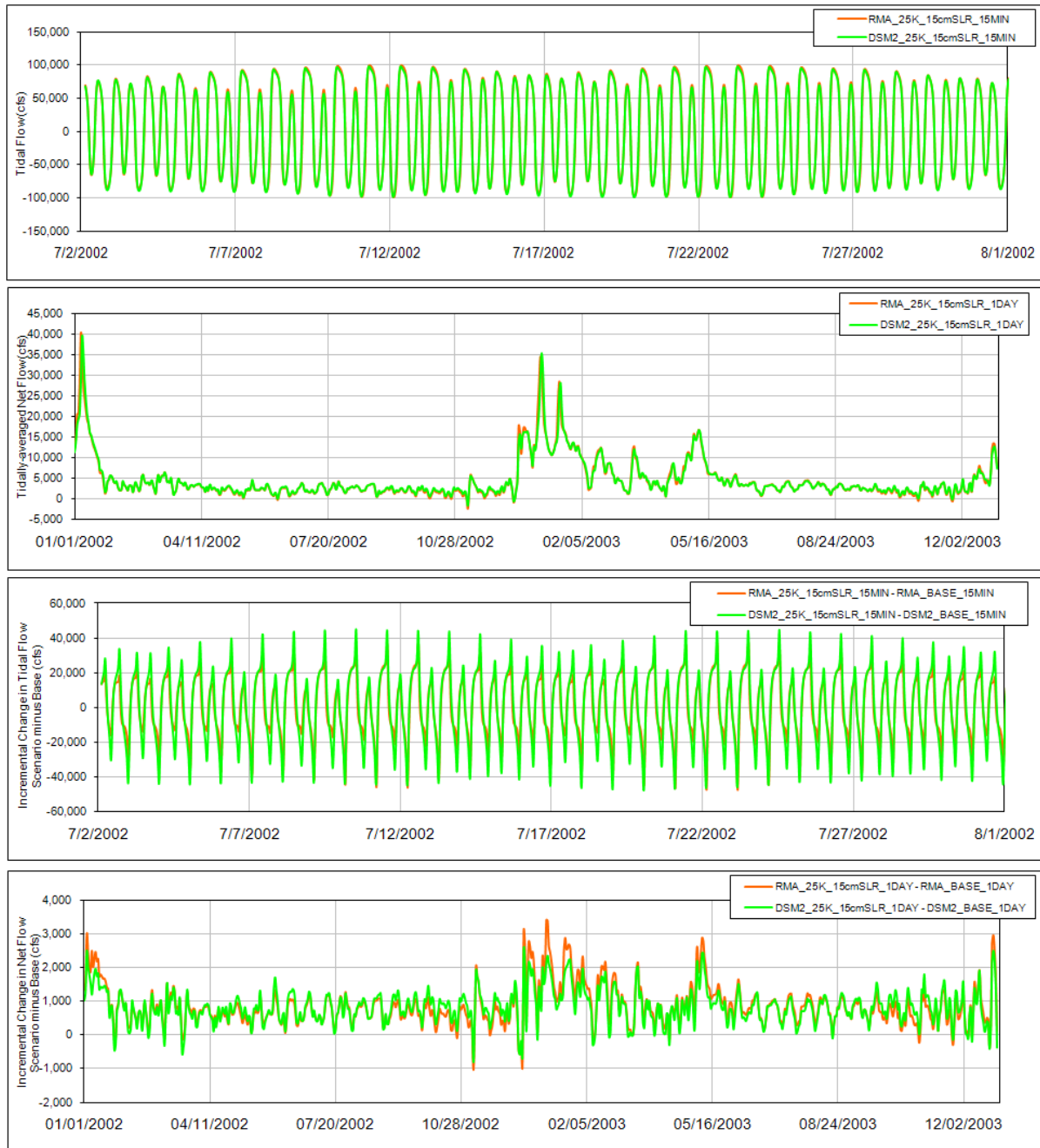
Figure 1-145. Comparison of Tidal Flow, Tidally-Averaged Daily Flow, Incremental Change in Tidal Flow and the Incremental Change in the Daily Flow between the Integrated Early Long-term Scenario and the Current Conditions Scenario from RMA Model and DSM2 Model for Cache Slough at Ryer Island Location.
