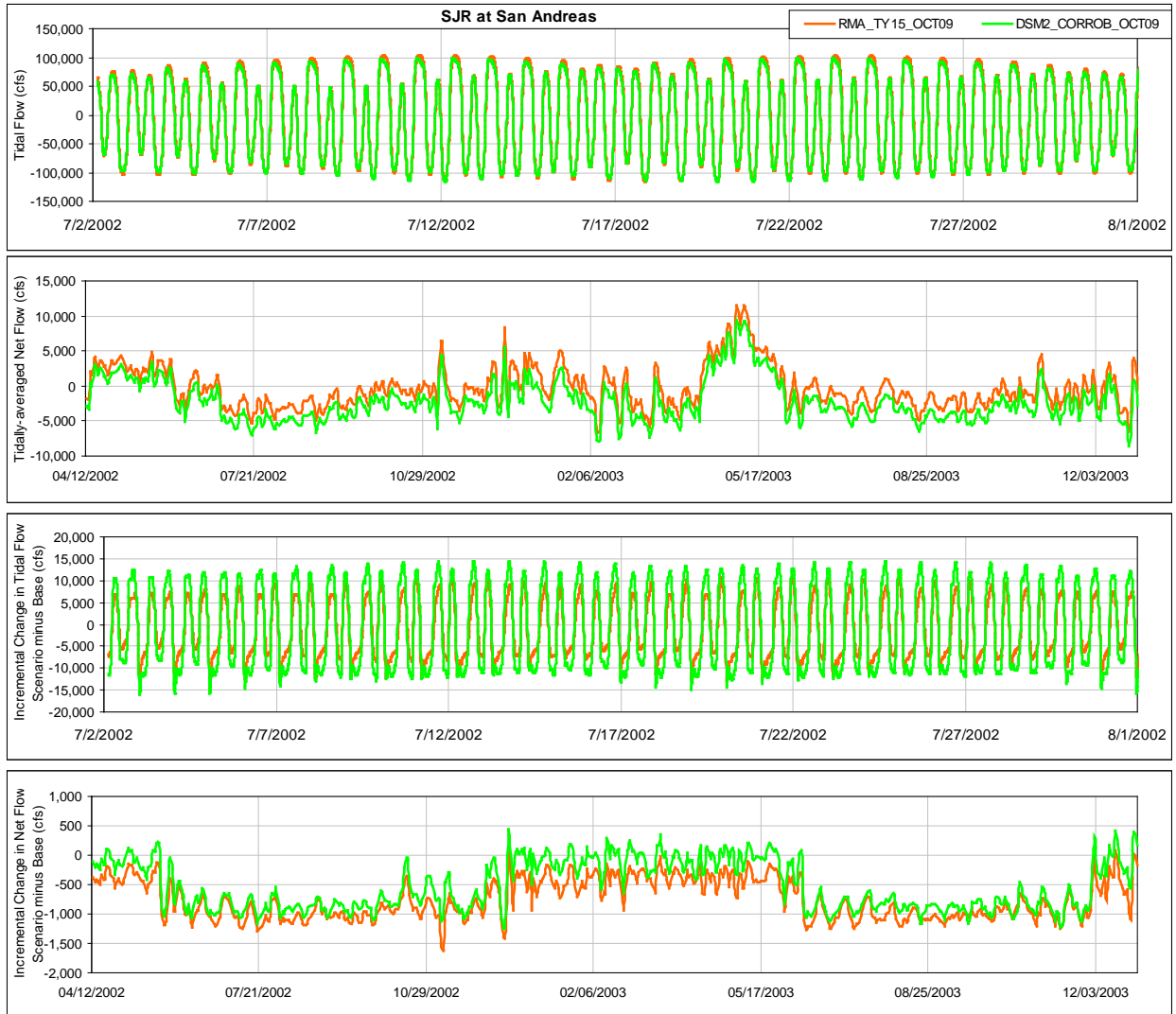
1 Figure 1-50. Comparison of Tidal Flow, Tidally-Averaged Daily Flow, Incremental Change in Tidal 2 Flow and the Incremental Change in the Daily Flow between the Early Long-term Scenario and the 3 Current Conditions Scenario from RMA Model and DSM2 Model for San Joaquin River at San 4 Andreas Location
