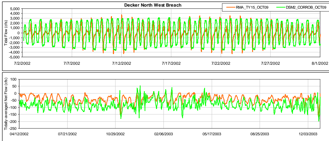
1 Figure 1-62. Comparison of Tidal Flow, Tidally-Averaged Daily Flow between the Early Long-Term 2 Scenario and the Current Conditions Scenario from RMA Model and DSM2 Model for Decker Island 3 North West Breach under West Delta Region
