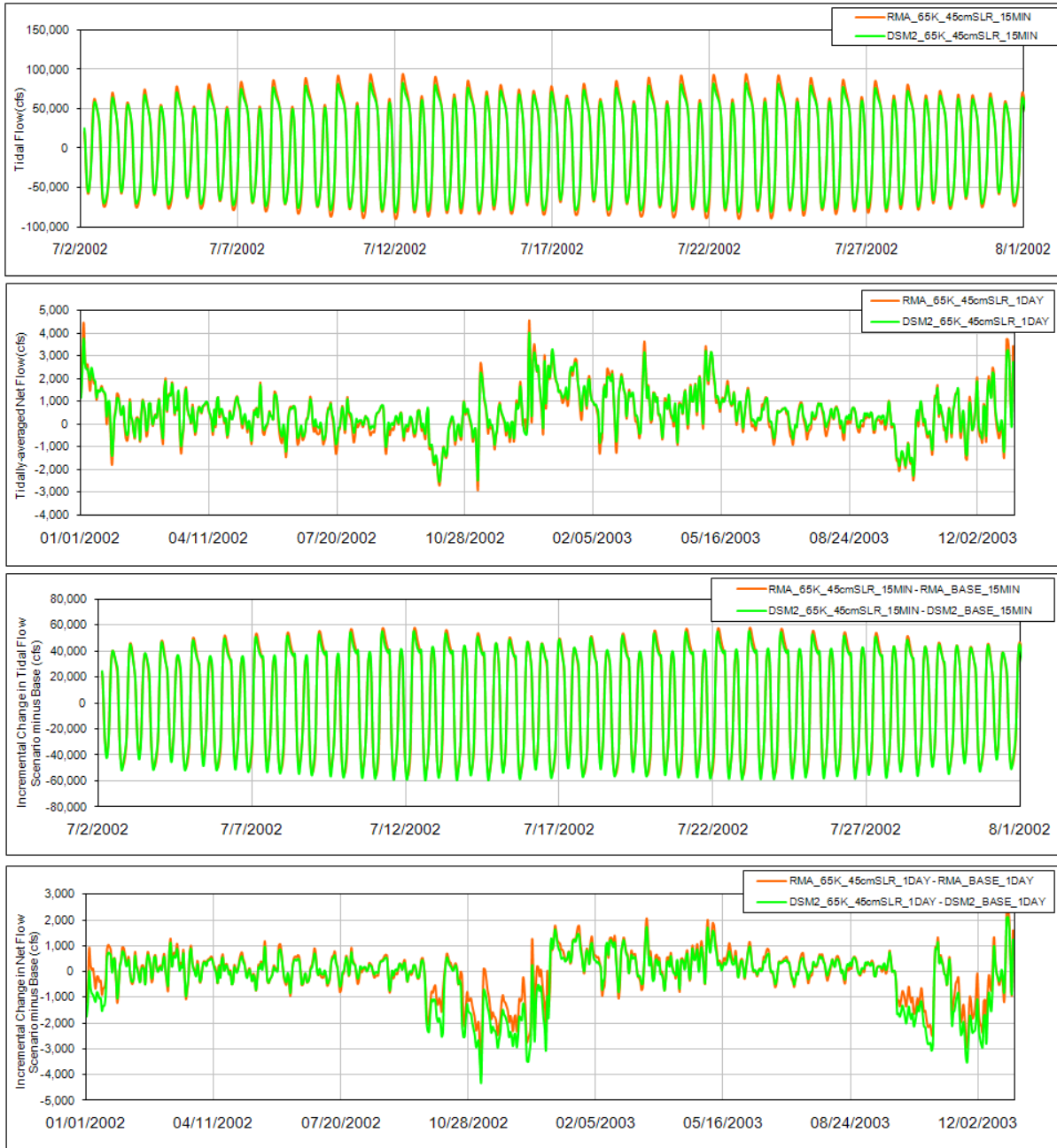
1 Figure 1-193. Comparison of Tidal Flow, Tidally-Averaged Daily Flow, Incremental Change in Tidal Flow 2 and the Incremental Change in the Daily Flow between the Integrated Late Long-term Scenario and the 3 Current Conditions Scenario from RMA Model and DSM2 Model for Montezuma Slough at Mouth 4 Location. 5
