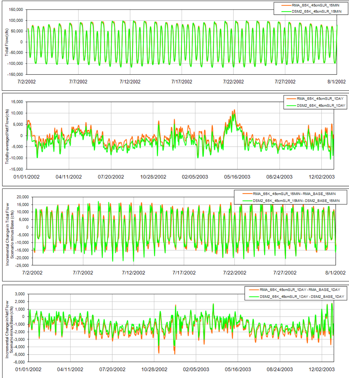
1 2 Figure 48: Comparison of Tidal Flow, Tidally-Averaged Daily Flow, Incremental Change in Tidal Flow 3 and the Incremental Change in the Daily Flow between the Integrated Late Long-term Scenario and 4 the Current Conditions Scenario from RMA Model and DSM2 Model for San Joaquin River at San 5 Andreas Location
