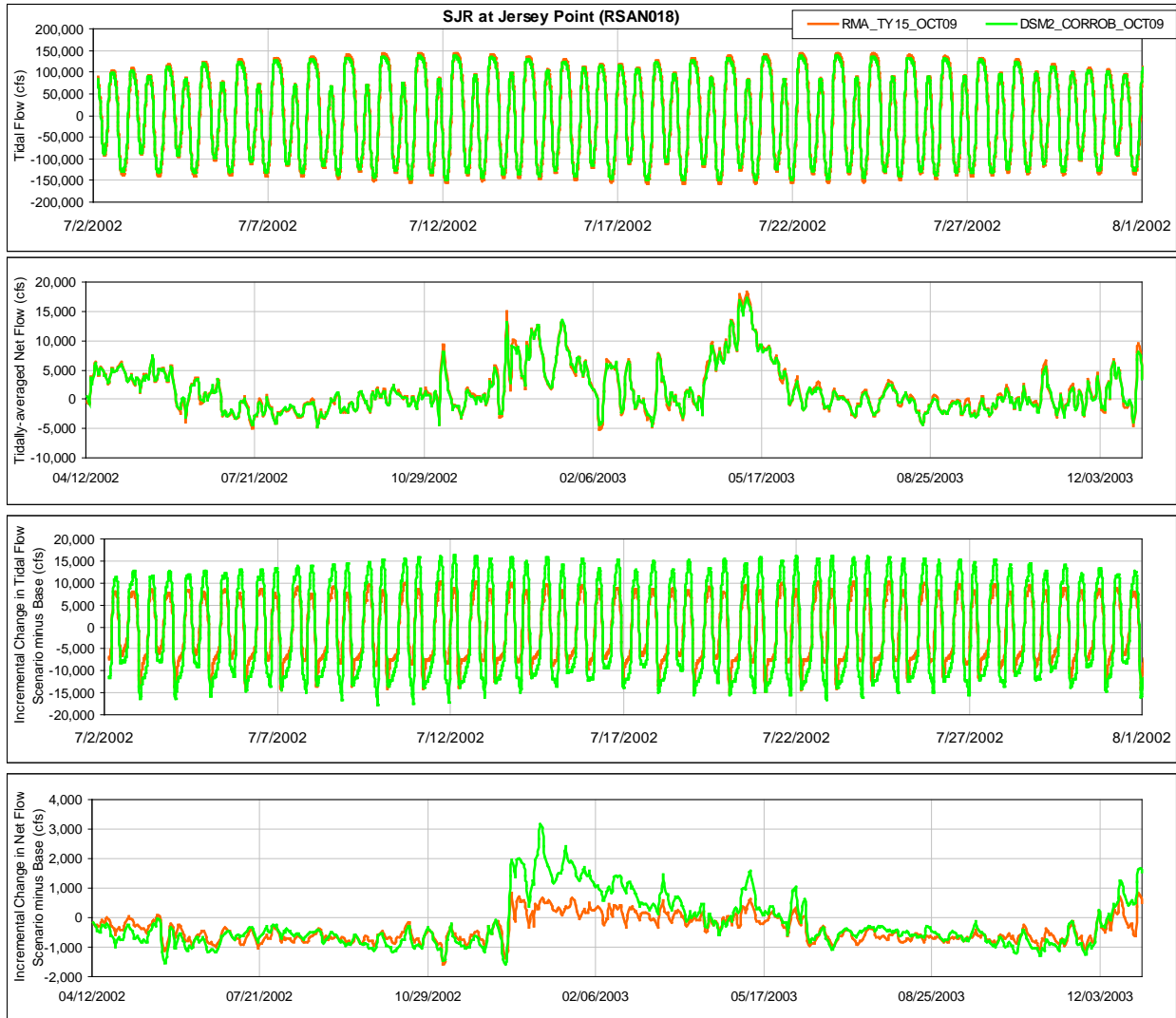
1 Figure 1-49. Comparison of Tidal Flow, Tidally-Averaged Daily Flow, Incremental Change in Tidal 2 Flow and the Incremental Change in the Daily Flow between the Early Long-term Scenario and the 3 Current Conditions Scenario from RMA Model and DSM2 Model for San Joaquin River at Jersey 4 Point Location
