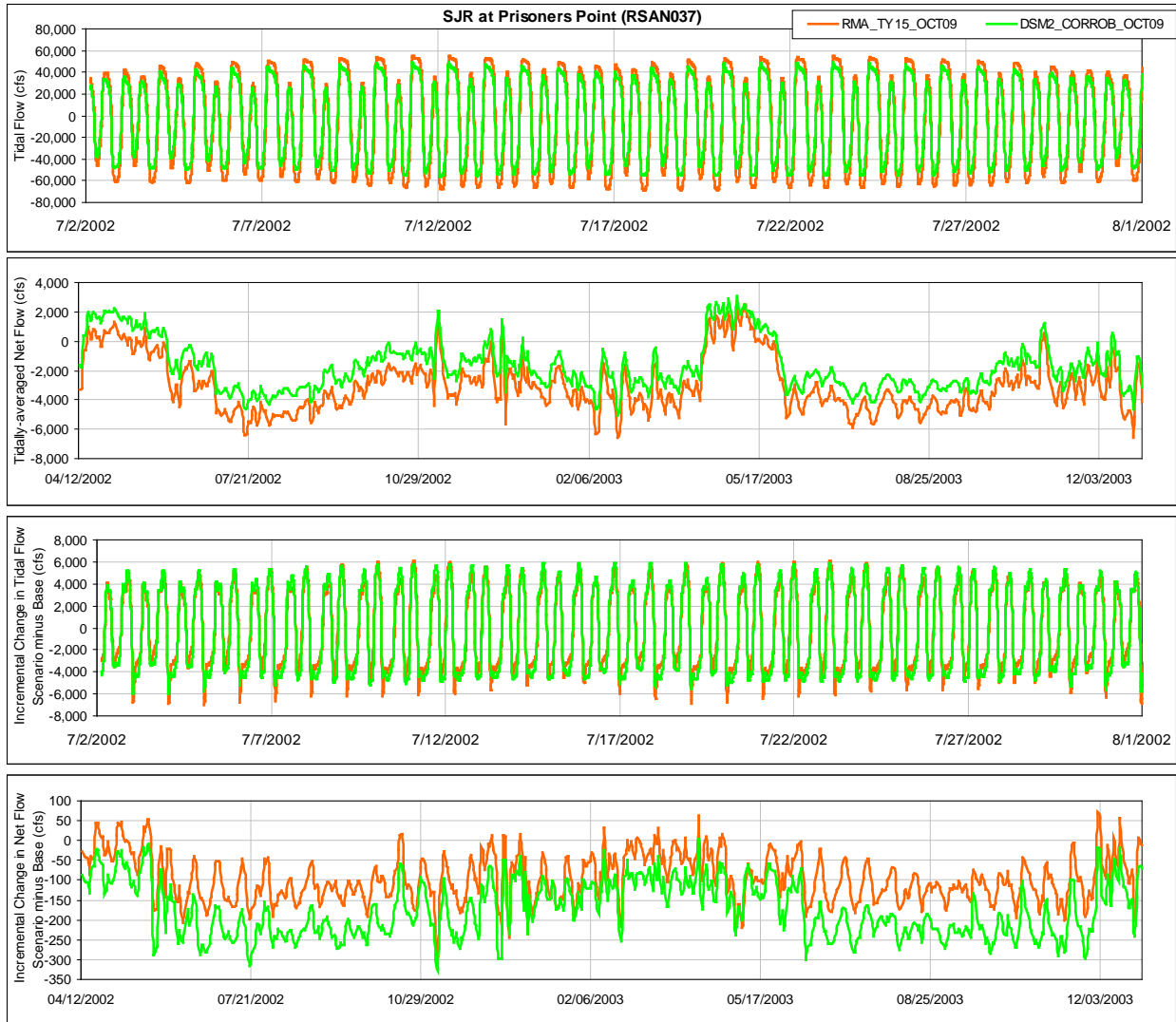
1 Figure 1-10. Comparison of Tidal Flow, Tidally-Averaged Daily Flow, Incremental Change in Tidal 2 Flow and the Incremental Change in the Daily Flow between the Near-Term Scenario and the 3 Current Conditions Scenario from RMA Model and DSM2 Model for San Joaquin River at Prisoners 4 Point Location
