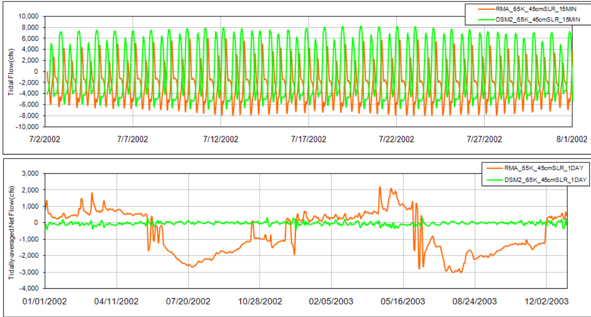
1 Figure 1-208. Comparison of Tidal Flow and Tidally-Averaged Daily Flow between the Integrated Late 2 Long-term Scenario and the Current Conditions Scenario from RMA Model and DSM2 Model for 3 Snodgrass Slough and McCormick Williamson Tract Breaches under Eastern Delta Region.
