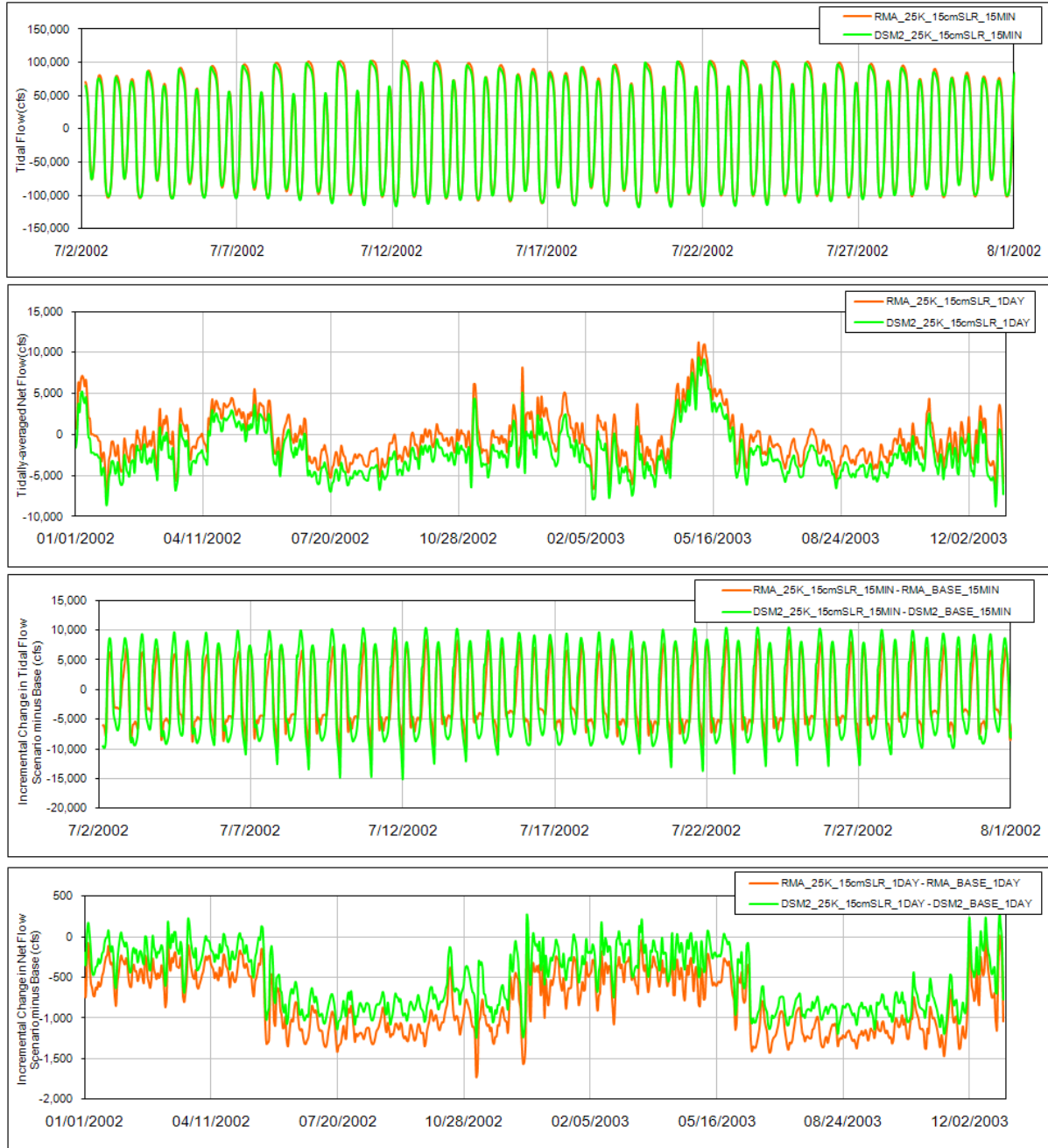
1 Figure 1-153. Comparison of Tidal Flow, Tidally-Averaged Daily Flow, Incremental Change in Tidal Flow 2 and the Incremental Change in the Daily Flow between the Integrated Early Long-term Scenario and the 3 Current Conditions Scenario from RMA Model and DSM2 Model for San Joaquin River at San Andreas 4 Location.
