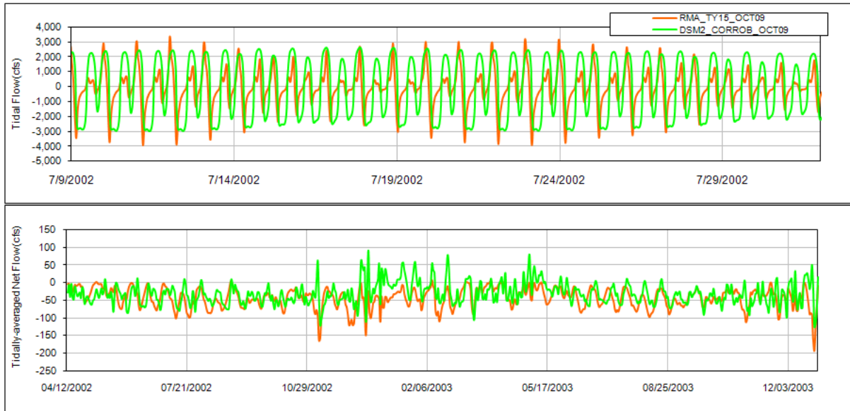
1 Figure 1-97. Comparison of Tidal Flow and Tidally-Averaged Daily Flow between the Late Long-Term 2 Scenario and the Current Conditions Scenario from RMA Model and DSM2 Model for Decker Island 3 North West Breach under Western Delta Region.
