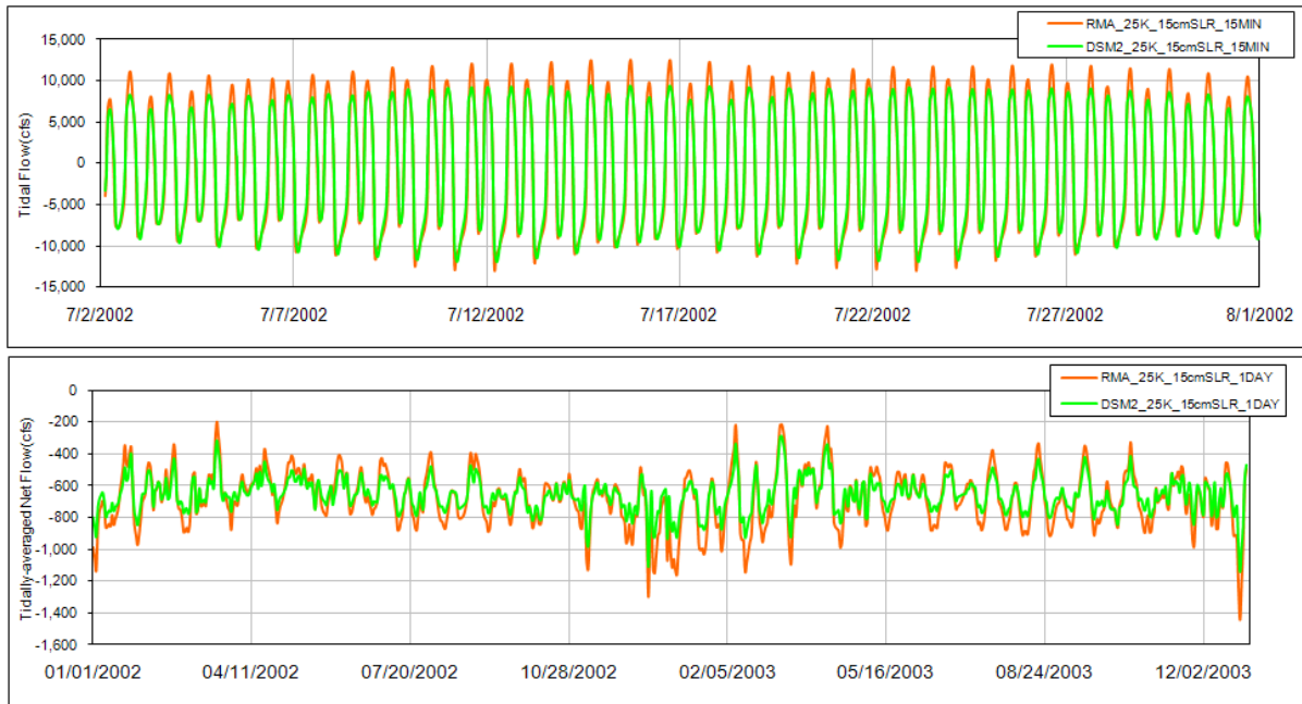
6 Figure 1-162. Comparison of Tidal Flow and Tidally-Averaged Daily Flow between the Integrated Early 7 Long-term Scenario and the Current Conditions Scenario from RMA Model and DSM2 Model for Suisun 8 Island 10 breach 3 under Suisun Marsh Region.
