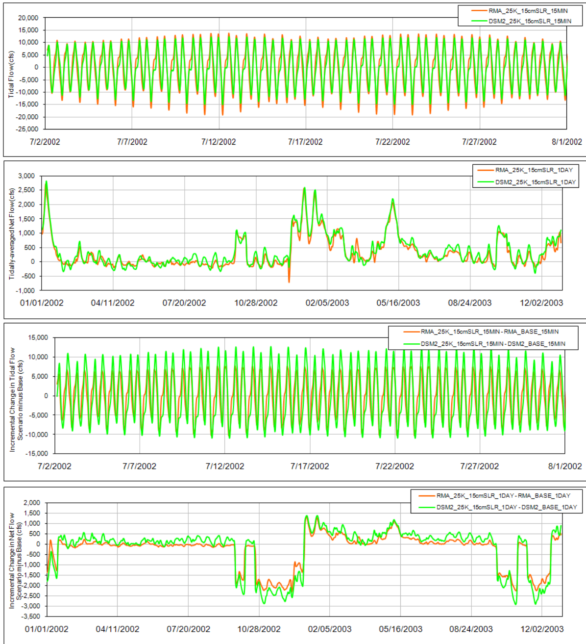
1 Figure 1-149. Comparison of Tidal Flow, Tidally-Averaged Daily Flow, Incremental Change in Tidal Flow 2 and the Incremental Change in the Daily Flow between the Integrated Early Long-term Scenario and the 3 Current Conditions Scenario from RMA Model and DSM2 Model for Montezuma Slough at Head Location. 4
