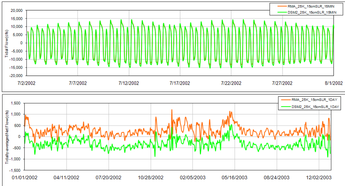
6 Figure 1-166. Comparison of Tidal Flow and Tidally-Averaged Daily Flow between the Integrated Early 7 Long-term Scenario and the Current Conditions Scenario from RMA Model and DSM2 Model for Dutch 8 Slough d/s of Emerson Slough under Western Delta Region.
