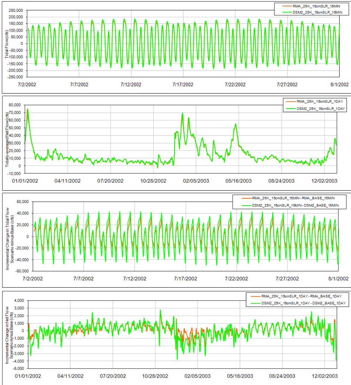
Figure 1-148. Comparison of Tidal Flow, Tidally-Averaged Daily Flow, Incremental Change in Tidal Flow and the Incremental Change in the Daily Flow between the Integrated Early Long-term Scenario and the Current Conditions Scenario from RMA Model and DSM2 Model for Sacramento River at Emmaton Location.
