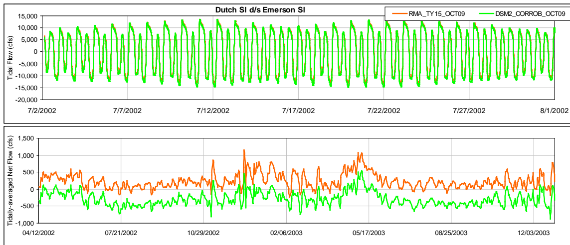
5 Figure 1-63. Comparison of Tidal Flow, Tidally-Averaged Daily Flow between the Early Long-Term 6 Scenario and the Current Conditions Scenario from RMA Model and DSM2 Model for Dutch SI d/s 7 Emerson SI under West Delta Region
