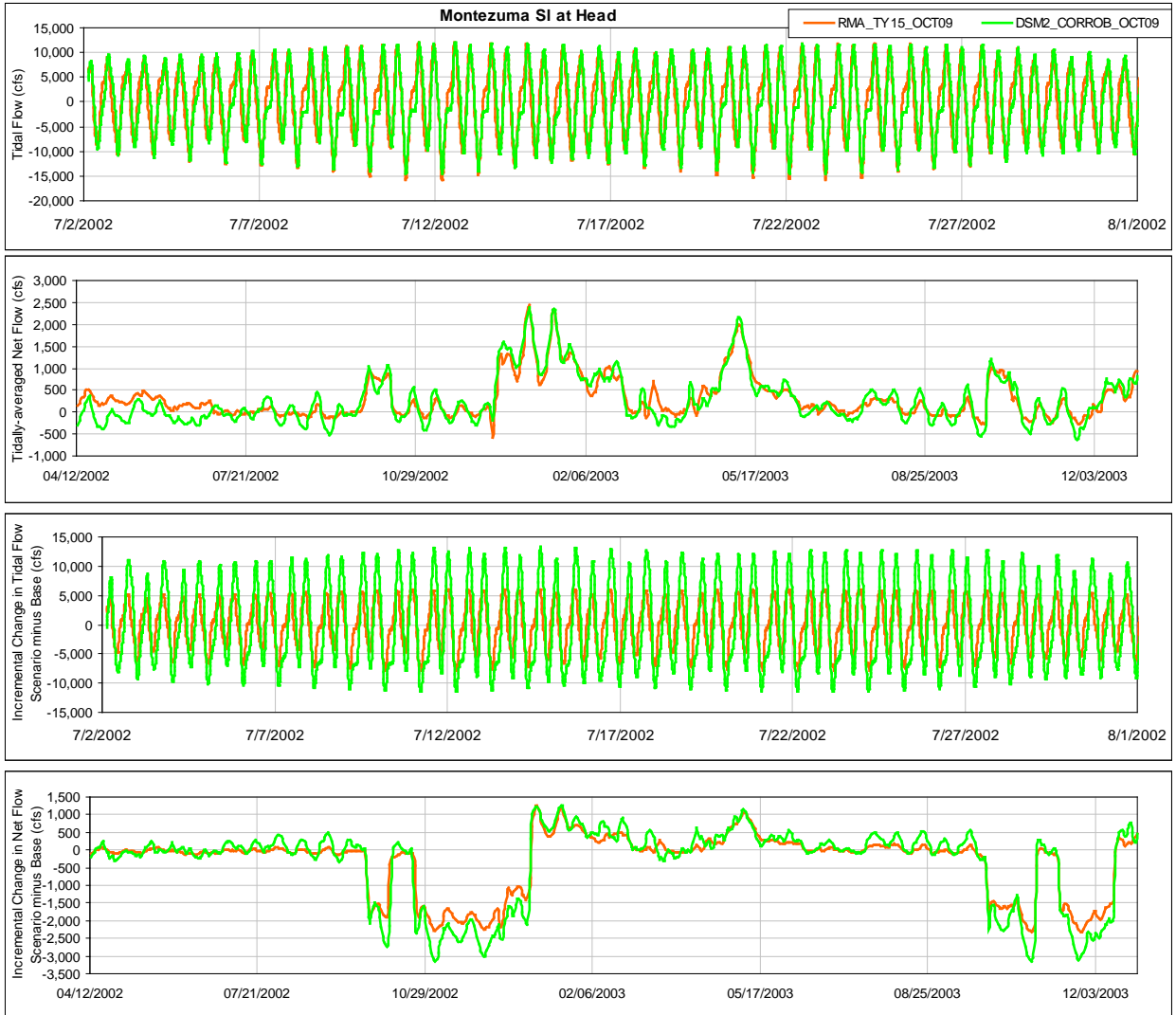
1 Figure 1-46. Comparison of Tidal Flow, Tidally-Averaged Daily Flow, Incremental Change in Tidal 2 Flow and the Incremental Change in the Daily Flow between the Early Long-term Scenario and the 3 Current Conditions Scenario from RMA Model and DSM2 Model for Montezuma SI at Head Location
