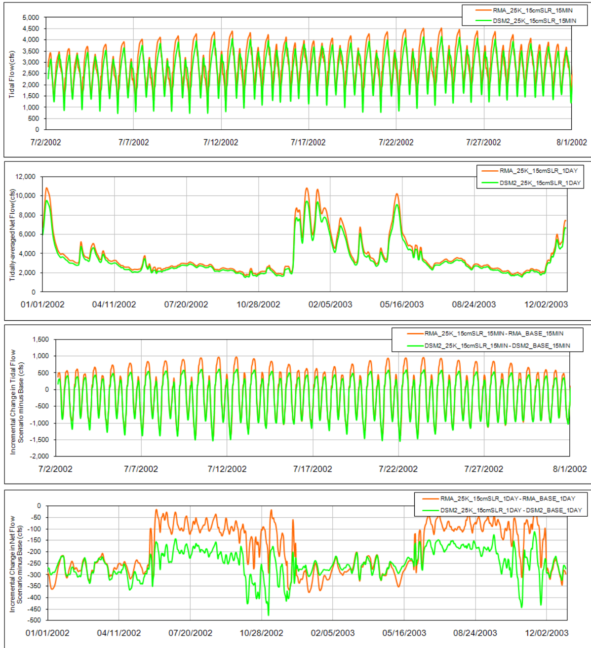
Figure 1-147. Comparison of Tidal Flow, Tidally-Averaged Daily Flow, Incremental Change in Tidal Flow and the Incremental Change in the Daily Flow between the Integrated Early Long-term Scenario and the Current Conditions Scenario from RMA Model and DSM2 Model for Georgiana Slough at Head Location.
