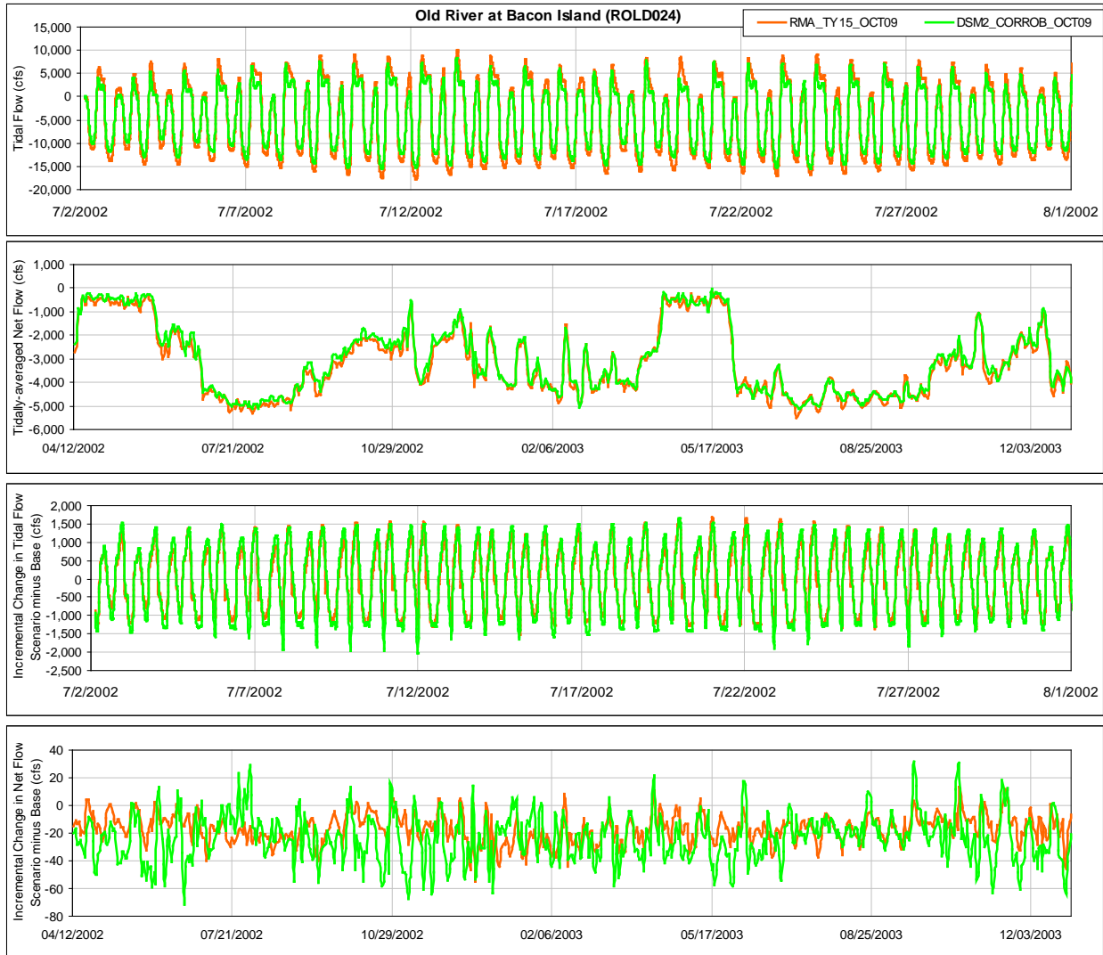
1 Figure 1-55. Comparison of Tidal Flow, Tidally-Averaged Daily Flow, Incremental Change in Tidal 2 Flow and the Incremental Change in the Daily Flow between the Early Long-term Scenario and the 3 Current Conditions Scenario from RMA Model and DSM2 Model for Old River at Bacon Island 4 Location
