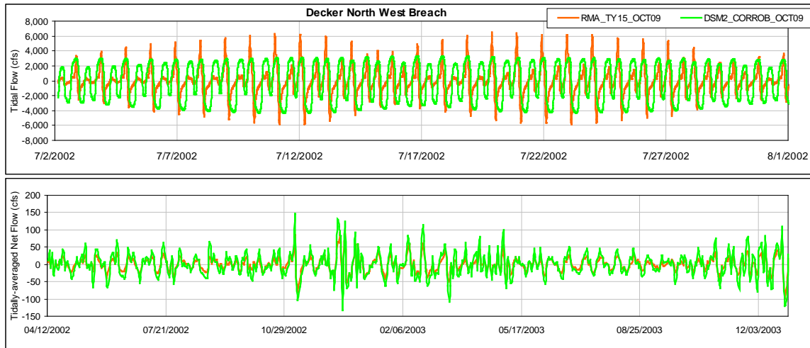
5 6 Figure 1-22. Comparison of Tidal Flow, Tidally-Averaged Daily Flow, Incremental Change in Tidal 7 Flow and the Incremental Change in the Daily Flow between the Near-Term Scenario and the 8 Current Conditions Scenario from RMA Model and DSM2 Model for Dutch SI d/s of Emerson SI 9 under West Delta Region
