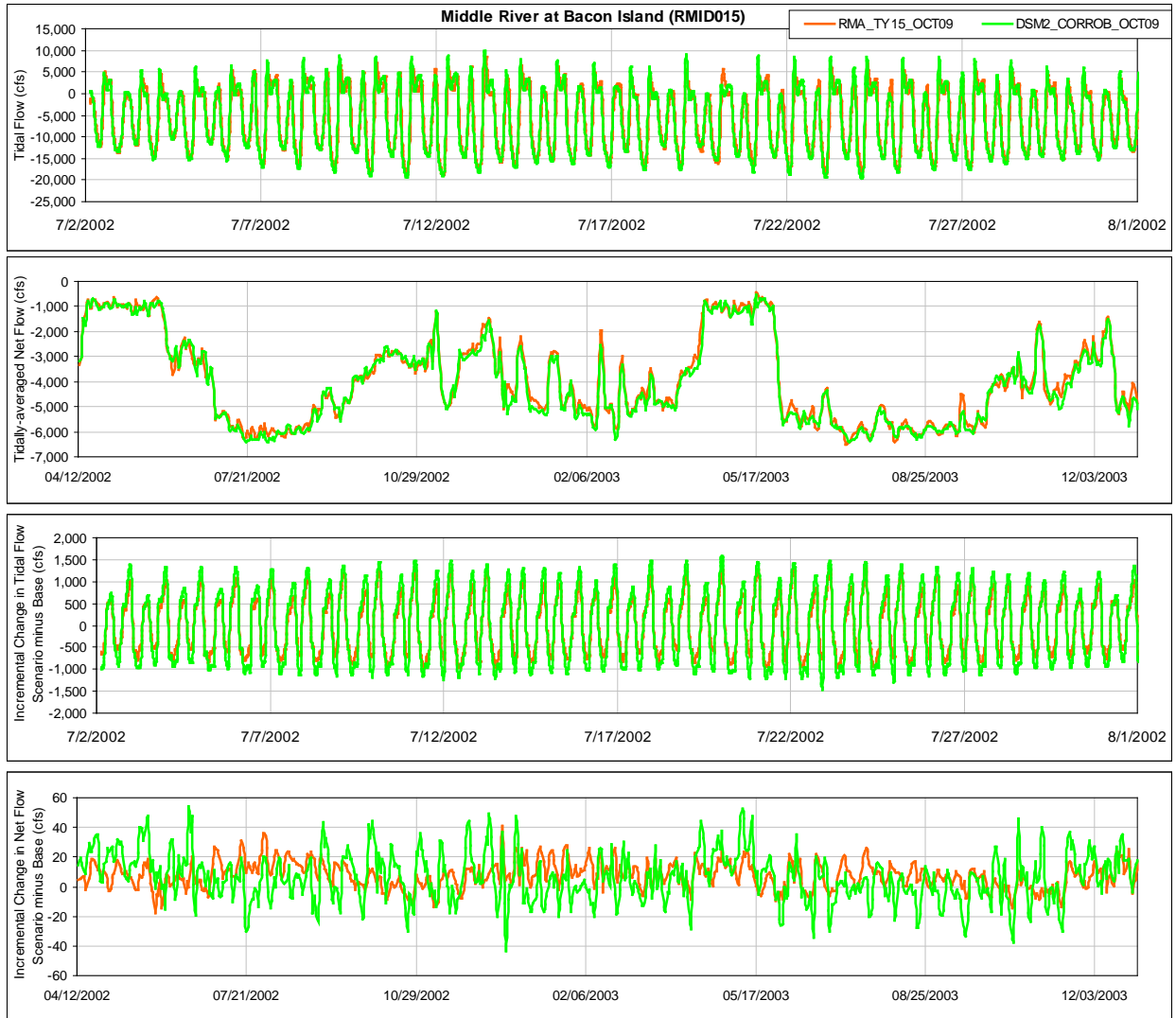
1 Figure 1-13. Comparison of Tidal Flow, Tidally-Averaged Daily Flow, Incremental Change in Tidal 2 Flow and the Incremental Change in the Daily Flow between the Near-Term Scenario and the 3 Current Conditions Scenario from RMA Model and DSM2 Model for Middle River at Bacon Island 4 Location
