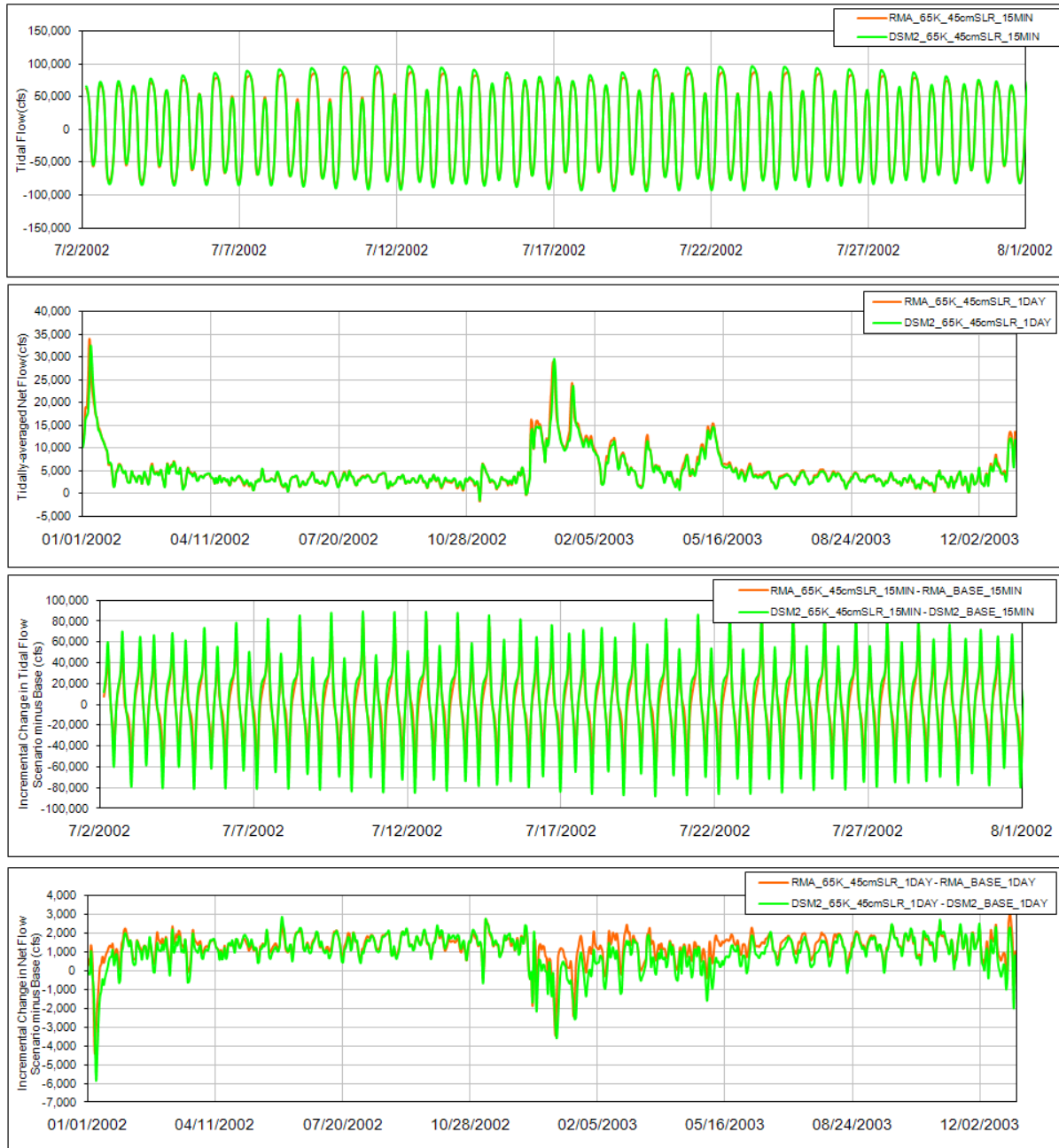
Figure 1-189. Comparison of Tidal Flow, Tidally-Averaged Daily Flow, Incremental Change in Tidal Flow and the Incremental Change in the Daily Flow between the Integrated Late Long-term Scenario and the Current Conditions Scenario from RMA Model and DSM2 Model for Cache at Ryer Island Location.
