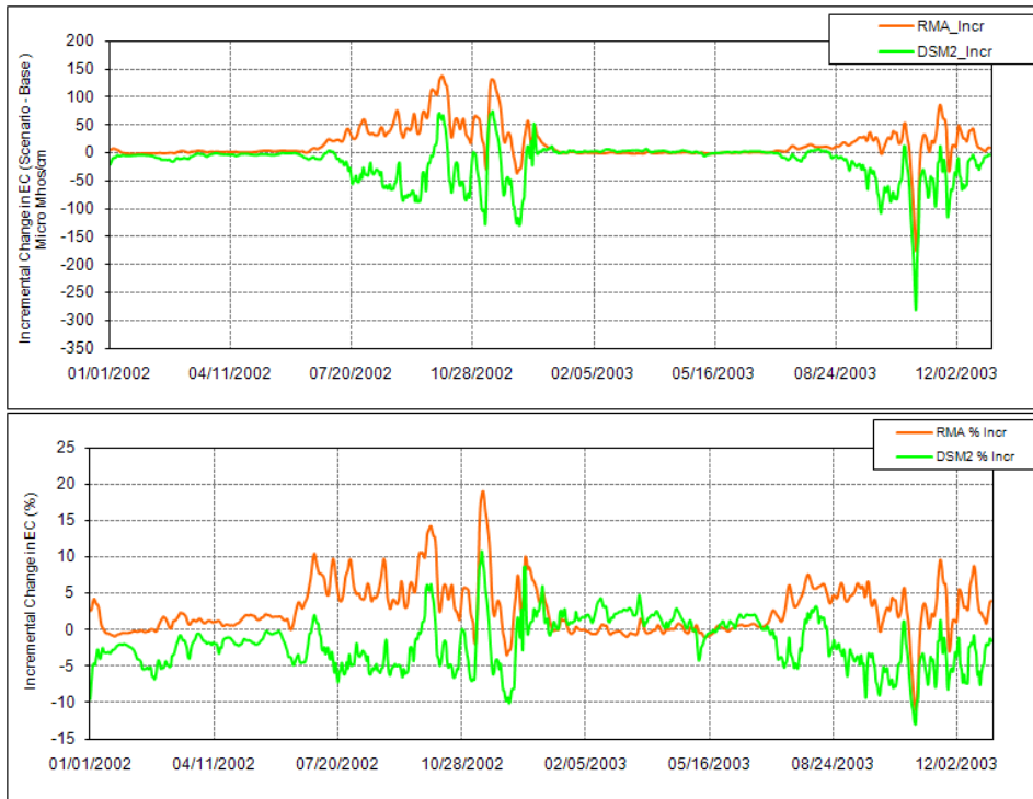
4 5 Figure 1-181. Comparison of Tidally-Averaged Daily EC and the Incremental Change in the Daily EC 6 between the Integrated Early Long-Term Scenario and the Current Conditions Scenario from RMA Model 7 and DSM2 Model for Three Mile Slough at San Joaquin River Location.
