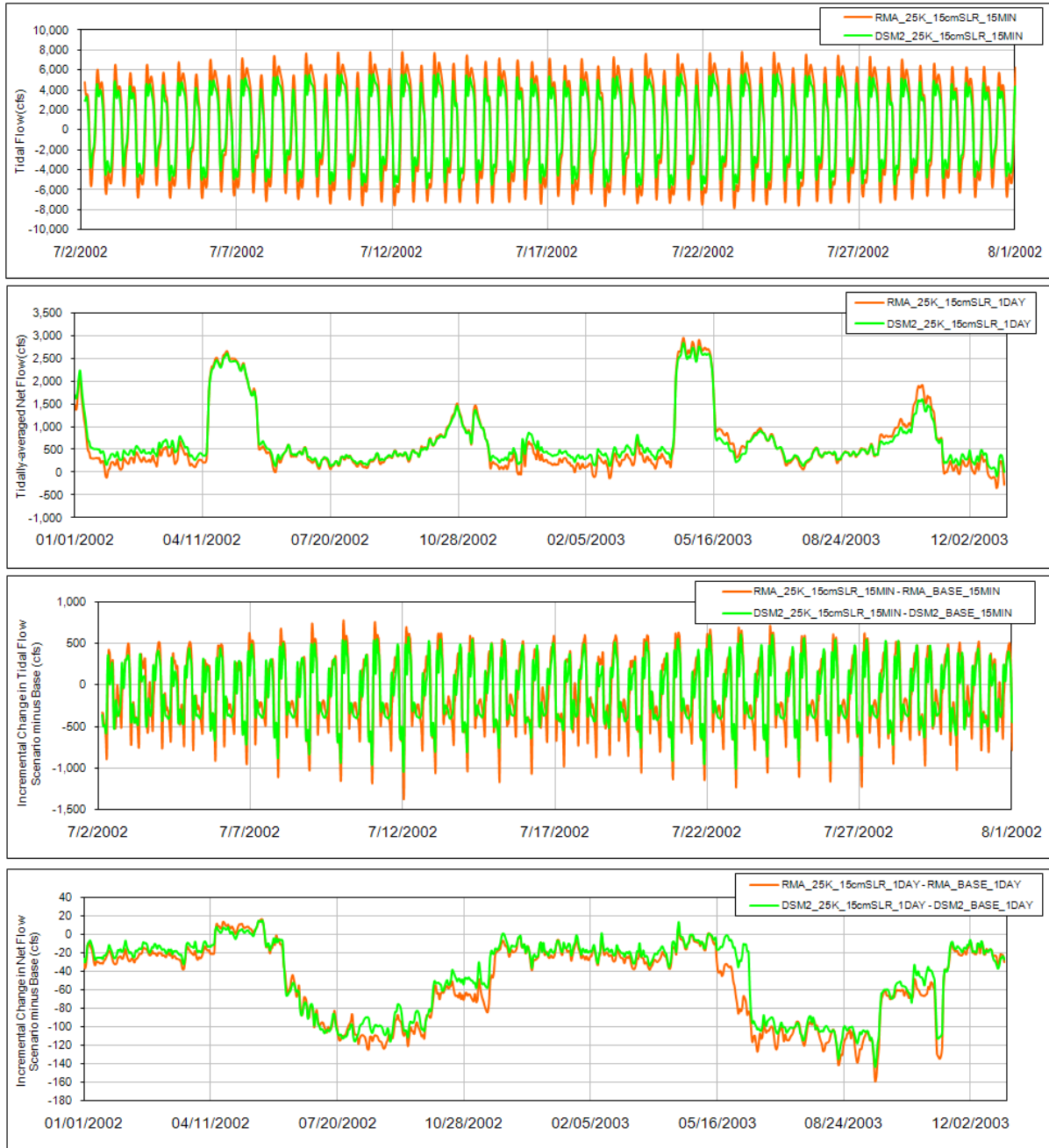
1 Figure 1-155. Comparison of Tidal Flow, Tidally-Averaged Daily Flow, Incremental Change in Tidal Flow 2 and the Incremental Change in the Daily Flow between the Integrated Early Long-term Scenario and the 3 Current Conditions Scenario from RMA Model and DSM2 Model for San Joaquin River at Stockton 4 Location. 5
