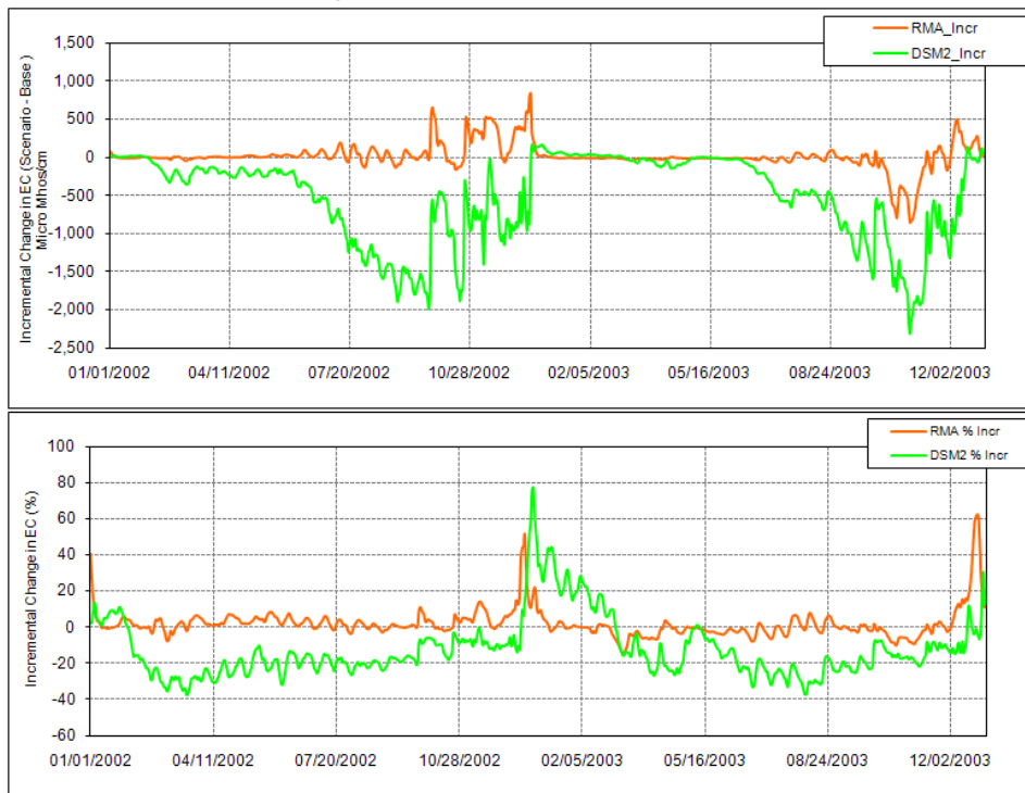
4 5 Figure 1-175. Comparison of Tidally-Averaged Daily EC and the Incremental Change in the Daily EC 6 between the Integrated Early Long-Term Scenario and the Current Conditions Scenario from RMA Model 7 and DSM2 Model for Montezuma Slough at Head Location.
