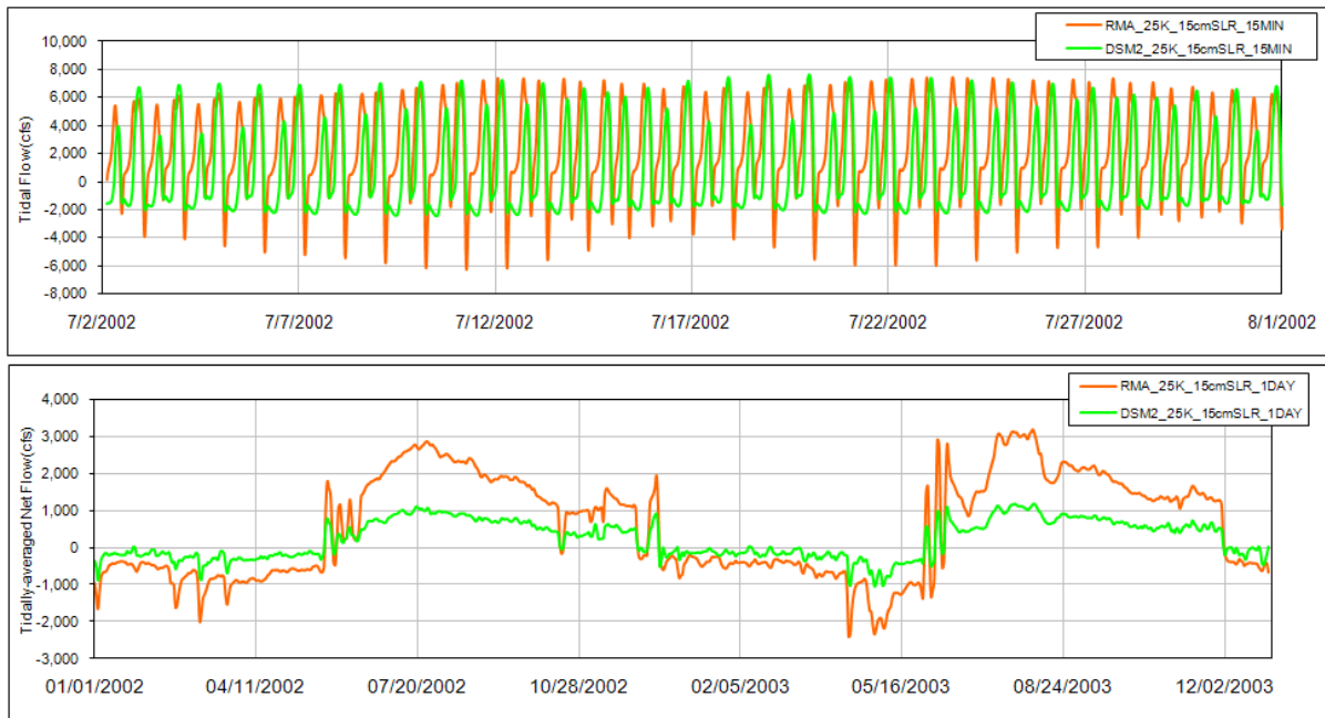
5 6 Figure 1-168. Comparison of Tidal Flow and Tidally-Averaged Daily Flow between the Integrated Early 7 Long-term Scenario and the Current Conditions Scenario from RMA Model and DSM2 Model for 8 Snodgrass Slough south and McCormick Williamson Tract breaches under Eastern Delta Region. 9
