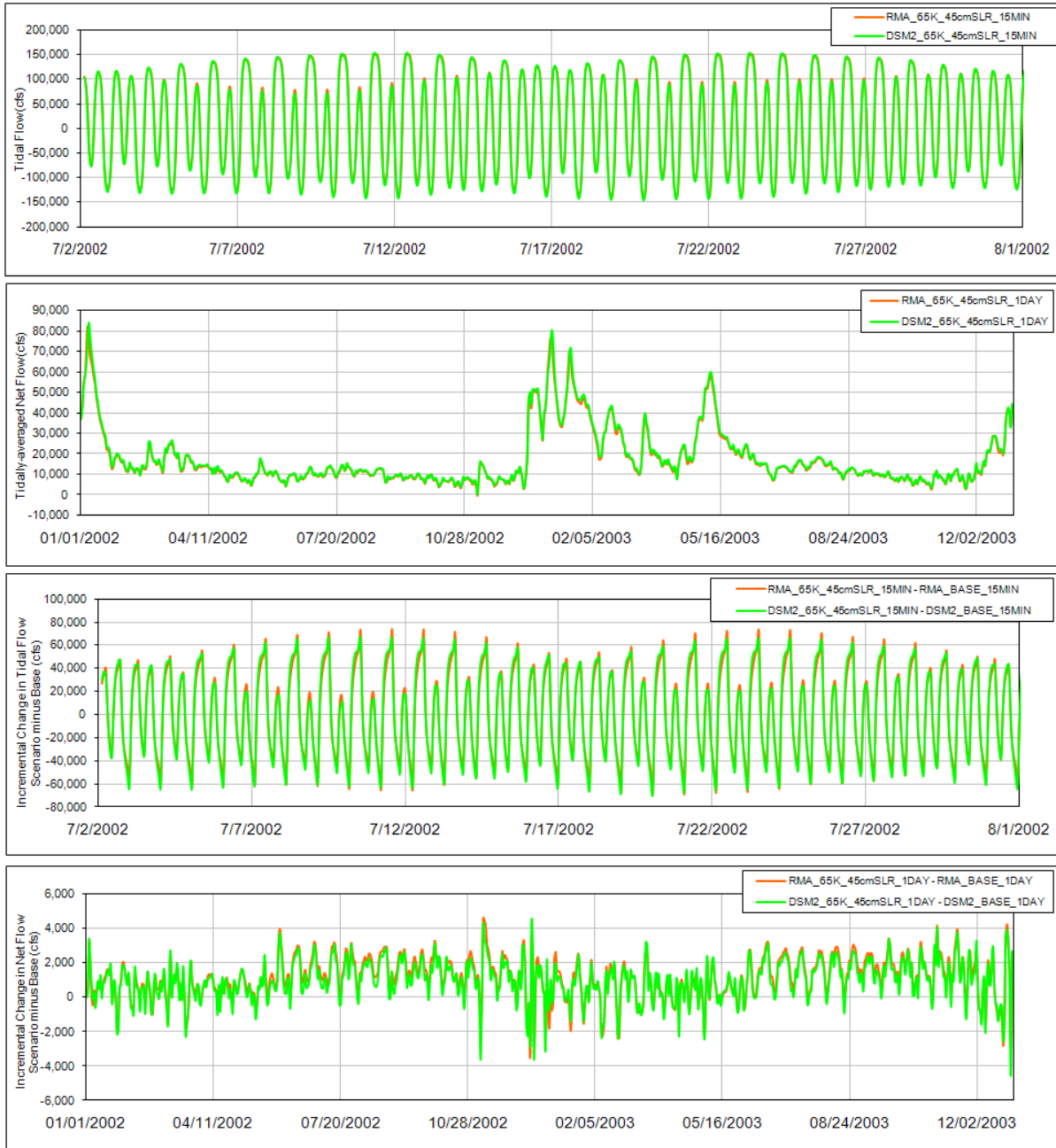
1 Figure 1-190. Comparison of Tidal Flow, Tidally-Averaged Daily Flow, Incremental Change in Tidal Flow 2 and the Incremental Change in the Daily Flow between the Integrated Late Long-term Scenario and the 3 Current Conditions Scenario from RMA Model and DSM2 Model for Sacramento River at Rio Vista 4 Location. 5
