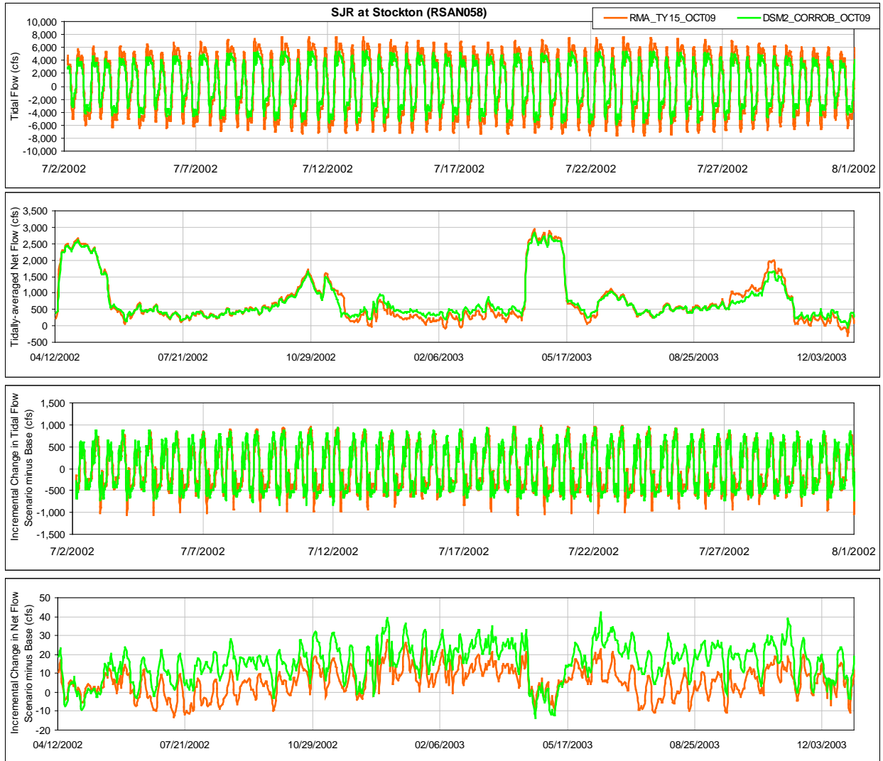
1 Figure 1-52. Comparison of Tidal Flow, Tidally-Averaged Daily Flow, Incremental Change in Tidal 2 Flow and the Incremental Change in the Daily Flow between the Early Long-term Scenario and the 3 Current Conditions Scenario from RMA Model and DSM2 Model for San Joaquin River at Stockton 4 Location
