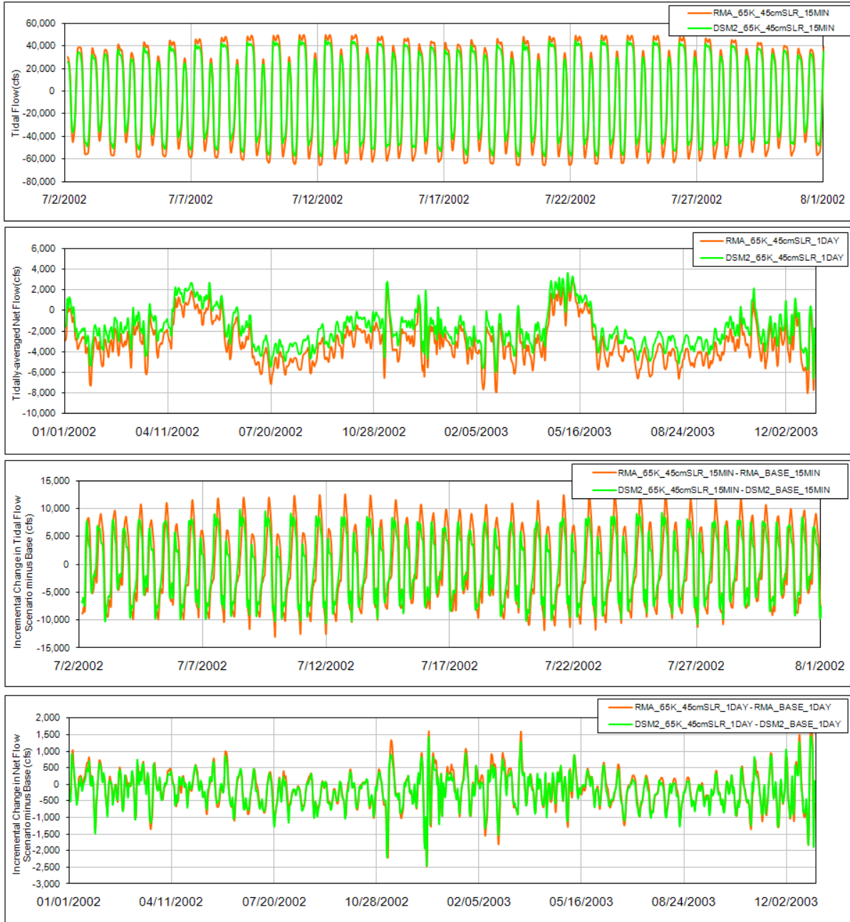
1 Figure 1-195. Comparison of Tidal Flow, Tidally-Averaged Daily Flow, Incremental Change in Tidal Flow 2 and the Incremental Change in the Daily Flow between the Integrated Late Long-term Scenario and the 3 Current Conditions Scenario from RMA Model and DSM2 Model for San Joaquin River at Prisoners Point 4 Location.
