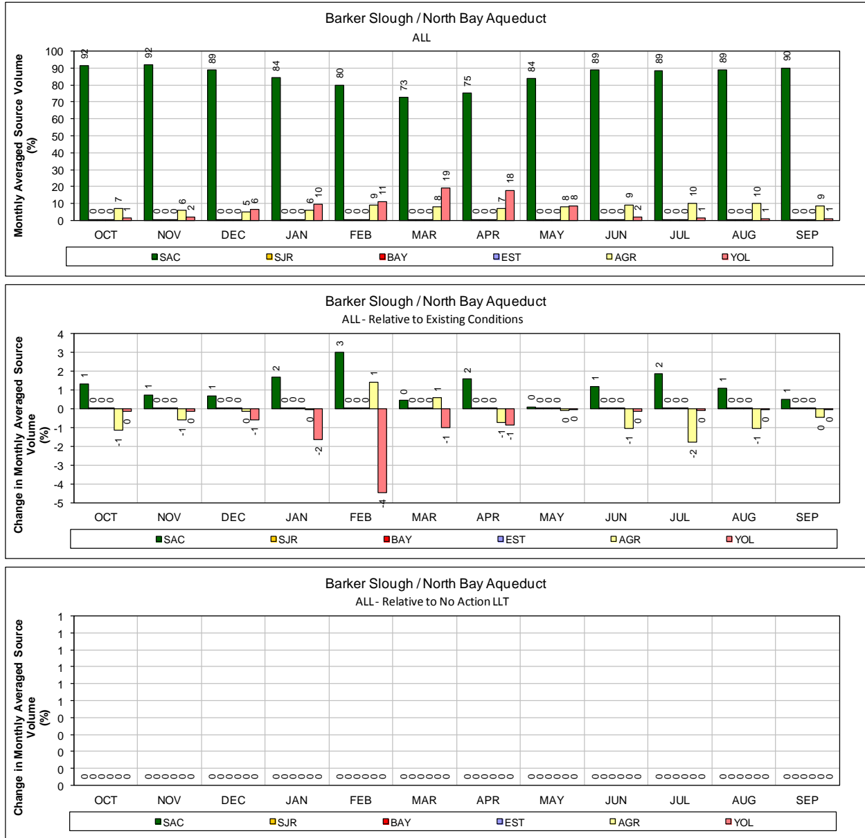
1 Figure 15.NA LLT – North Bay Aqueduct at Barker Slough Pumping Plant for ALL years (1976-1991) 2 Monthly average source volume (top figure) and change in monthly average source volume relative to 3 Existing Conditions and No Action Alternative Late Long Term (bottom two figures).
