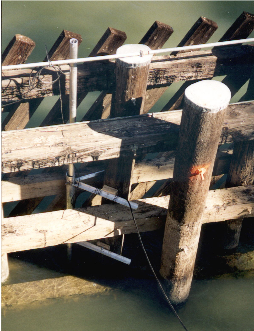
Figure 7. Typical mounting design for acoustic unit.
