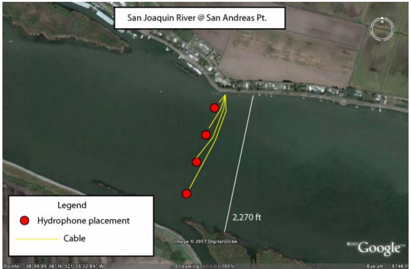
Figure 6.4 - Proposed 4-port system: hydrophone and communication cable locations in the San Joaquin River, at San Andreas Point (SAN). Exact hydrophone and cable locations will be determined through detailed field reconnaissance and testing conducted in the summer/fall of 2007.
