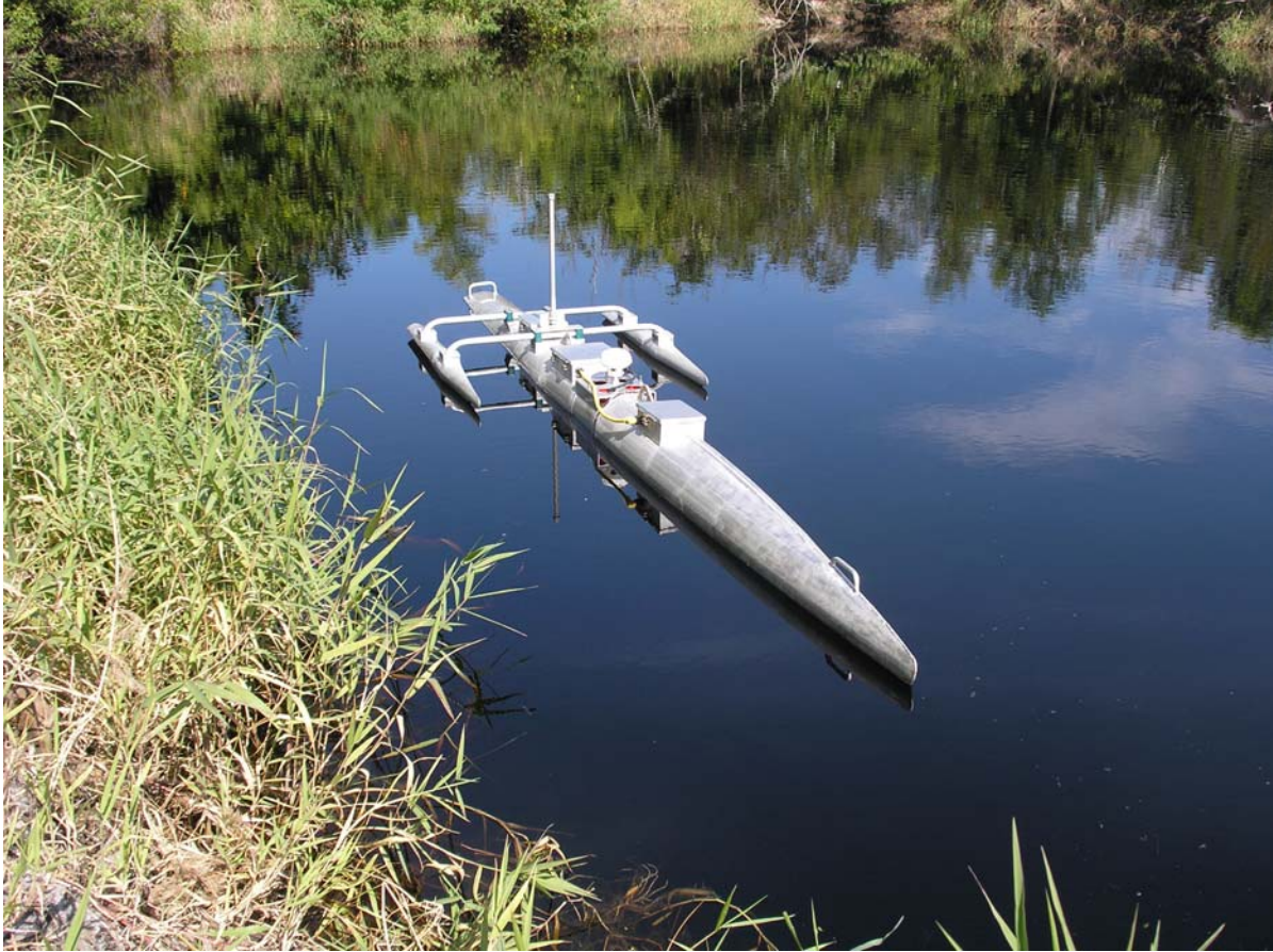
Figure 5.4 - SeaRobotics USV-1000 unmanned survey vessel, which will be used to collect detailed transects of the velocity structure upcurrent of the DCC and Georgiana Slough junctions.
