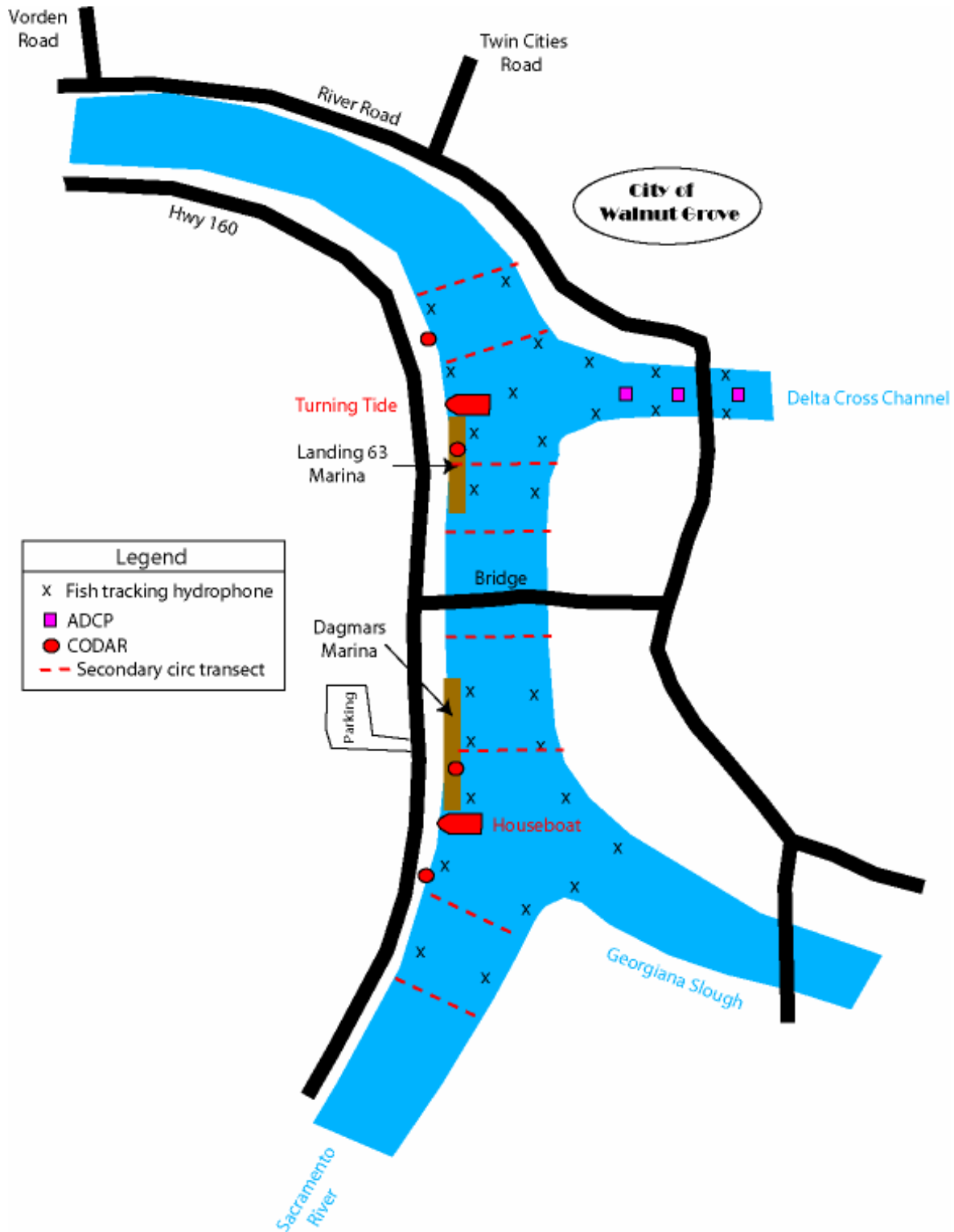
Figure 5.1 – Proposed experimental layout in the Sacramento River at junctions with the DCC and Georgiana Slough.
