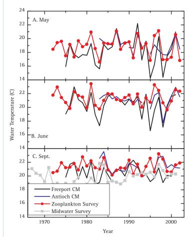
**Figure 18.** Monthly mean temperature in the Delta for selected months from two continuous monitoring (CM) sites (Freeport and Antioch) and two grab-sample sources (IEP zooplankton surveys and fall midwater trawl surveys for all Delta stations). Data from IEP web site.
