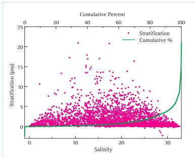
**Figure 24.** Salinity stratification vs. salinity from USGS monitoring data. Data are from 1988-2002 for 29 stations west of the Delta with at least 100 dates sampled. Water column mean salinity is averaged over all 1-m depth bins reported. Stratification is measured as the difference in salinity between 1 and 10 meters depth, or at least a 7-m depth range. The green line gives cumulative percent frequency of stratification.
