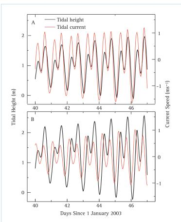
**Figure 9.** Example of tidal height (black lines, left axis) and tidal currents (red, right axis) for a single week. A., Carquinez Strait in the northern estuary; B., San Mateo Bridge in South Bay.
