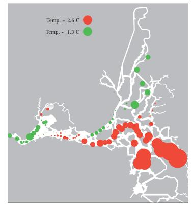
**Figure 19.** Spatial distribution of temperature in September in the Delta and Suisun Bay based on fall midwater trawl sample data. Each symbol represents the deviation from the spatially-averaged temperature for all years from 1990 to 2001 and for all stations sampled at least 7 times during that period.
