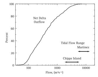
**Figure 14.** Frequency distribution of monthly net Delta outflow from DWR DAYFLOW program (line), with tidal volume fluxes for two locations shown as arrows connecting modeled values for spring and neap tides.
