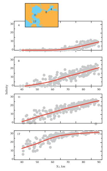
**Figure 22.** Salinity (practical salinity units) at four locations in the northern estuary plotted against X2. Data are from USGS monitoring stations shown on inset (Table 2). Data points are water column means of individual samples, and corresponding X2 value is for the same day. No tidal correction has been applied. Lines are from generalized additive models with smoothing splines fit to the data.
