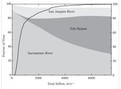
**Figure 5.** Proportion of inflow to the Delta from different sources based on monthly flow from water years 1956-2002 from the Dayflow program (http://iep.water.ca.gov/Dayflow). Remaining inflow is from small tributaries on the east side of the Delta (e.g., Mokelumne, Cosumnes). The black line is the cumulative percent frequency, i.e. the percent of inflow less than or equal to that value.
