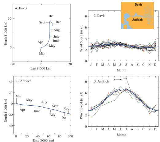
**Figure 15.** Wind conditions at Davis (16 years, data from Integrated Pest Management web site) and Antioch (7 years, DWR continuous monitoring site). A, B, progressive vector diagrams illustrate the mean daily wind at each location as a series of vectors resulting in the trajectory of a particle influenced by that wind speed and direction for one year. Letters indicate months. C, D, annual cycle of monthly mean wind speed at each location, with the grand mean shown by a heavy line.
