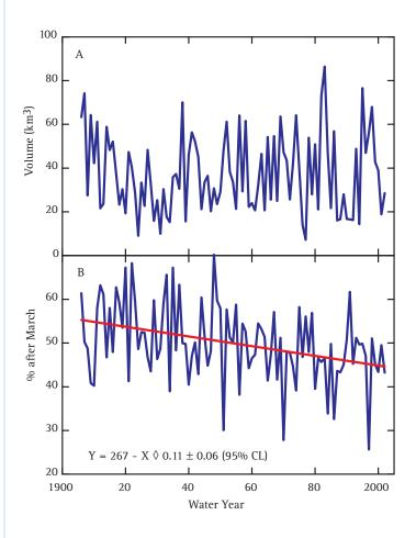
**Figure 3.** Estimated unimpaired flow for 1906-2002. A., Annual unimpaired flow calculated by regression from the Eight River Index on estimated unimpaired flow for 1921-1992 (DWR 1994): Unimp = -3.3 + 8River x  $1.38 \pm 0.016$  (95% CL), prediction MSE = 0.84 km<sup>3</sup>. B., Percent of total flow for water year that flowed after March, i.e., April through September. Red line is a significant linear regression (p < 0.001).
