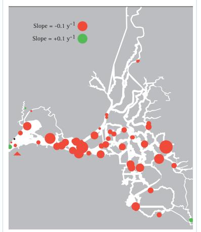
**Figure 28.** Spatial distribution of long-term change in turbidity. Data as in Figure 27B for individual stations, except that slopes of the long-term trends were calculated for each station by linear regression against year. Sizes of symbols indicate relative magnitude of the trend, and color indicates sign of trends significant at p< 0.05. Black symbols indicate no trend.
