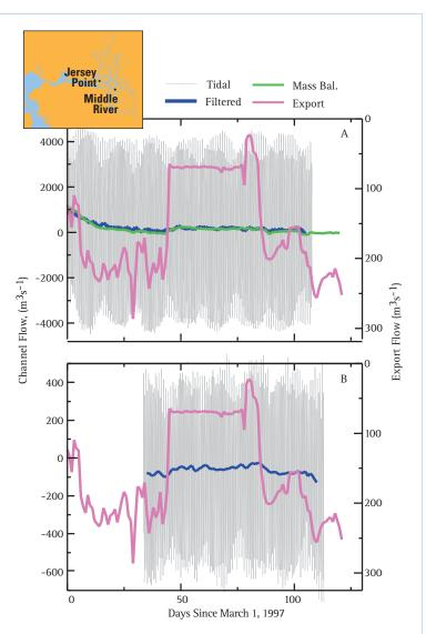
**Figure 21.** Flow patterns at two locations in the Delta in 1997 from USGS continuous montoring stations using ultrasonic velocity meters (Oltmann 1995, see Table 2). A, Jersey Point on the San Joaquin River; B, Middle River. Gray line, tidal flow data; blue line, tidally filtered data; green line, flow calculated by mass balance in the DWR Dayflow program (Jersey Point only, coded as QWEST); magenta line, export flow on a reversed scale.
