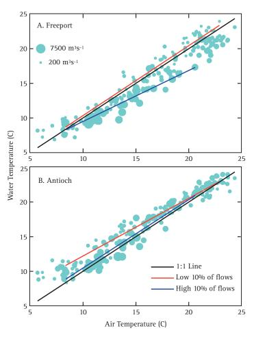
**Figure 17.** Monthly mean temperature at Freeport and Antioch vs. air temperature at Antioch. Size of symbols indicates freshwater flow. Lines are: Black = 1:1; Red: regression line for the lower 10th percentile of flow; Blue: regression line for upper 10th percentile of flow.
