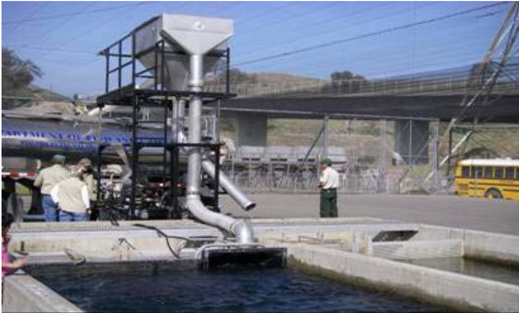
Figure 4-23. Aqua-Life Harvester Dewatering Tower loading juvenile steelhead.
