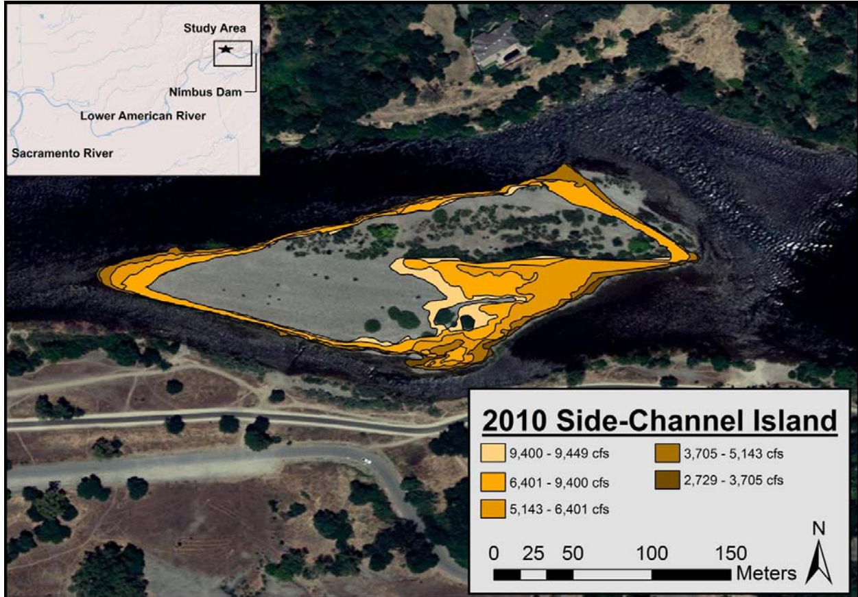
Figure 6. Current (post-2008–2010 gravel placement) areas of inundation for the side-channel island adjacent to the 2010 augmentation site. Flows ranged from 2,729 \text{ ft}^3 \cdot \text{s}^{-1} (23 February 2011) to 9,449 \text{ ft}^3 \cdot \text{s}^{-1} (4 January 2011). Color scale goes from dark to light (low flow to high flow). As flows increase, darker areas inundate first, followed by lighter areas. Visible areas represent exposed (i.e., non-inundated) floodplain.
