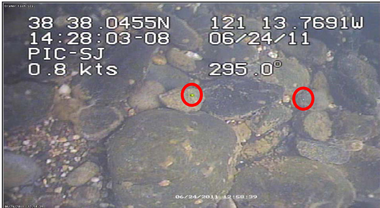
Figure 8. Example still shot taken during substrate surveys using underwater videography. Location of the still shot is displayed in the upper third of the frame. Lasers spaced at 6 inches (15.24 cm; circled in red) allowed us to use the ratio of each measured substrate sample to the measured known distance to calculate all substrate sample diameters. A horizontal transect line would be placed across the middle of each still shot, and the diameters of the first 10 substrate samples (i.e., individual pebble or piece of gravel) along the line would be measured.
