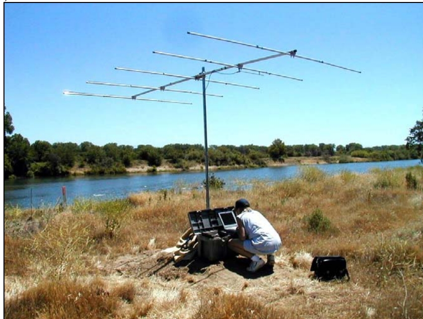
Figure 4. Fixed-station electronic data logger used in the fish radio-telemetry studies. Station shown was placed downstream of the gradient facility (mid-island).
