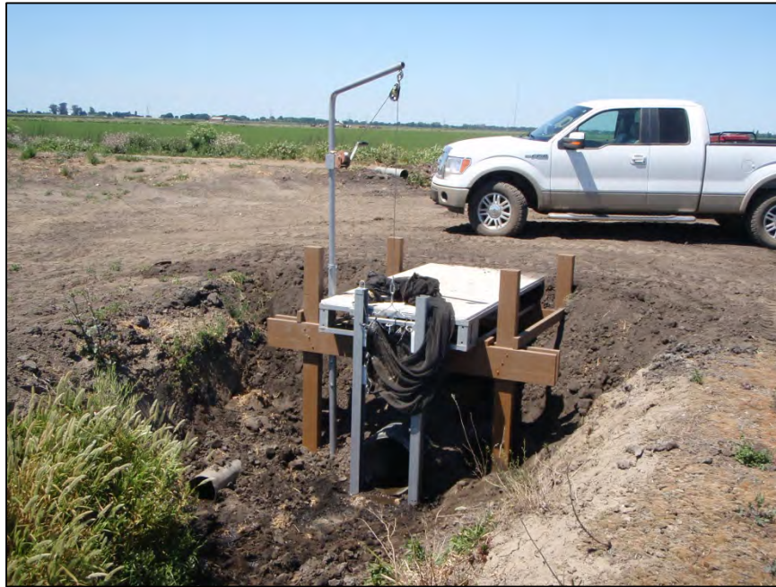
Figure 15. The fyke net, sampling platform, and associated apparatus used to sample for fish entrainment in the Sanchez east canal.
