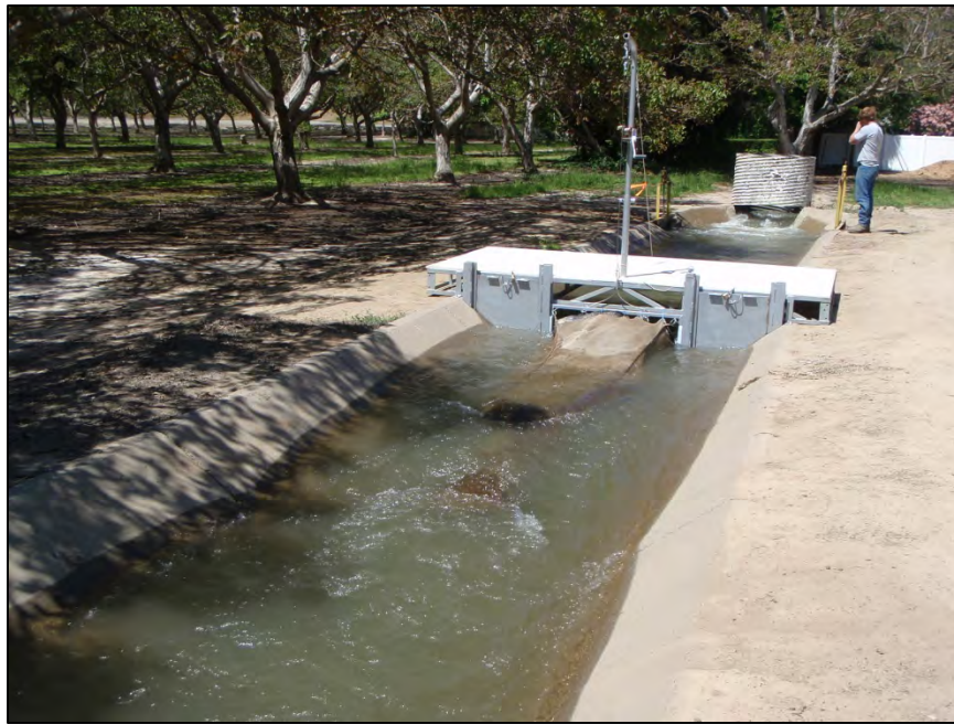
Figure 10. The fyke net, sampling platform, and associated apparatus used to sample for fish entrainment in the Alamo trapezoidal concrete canal.
