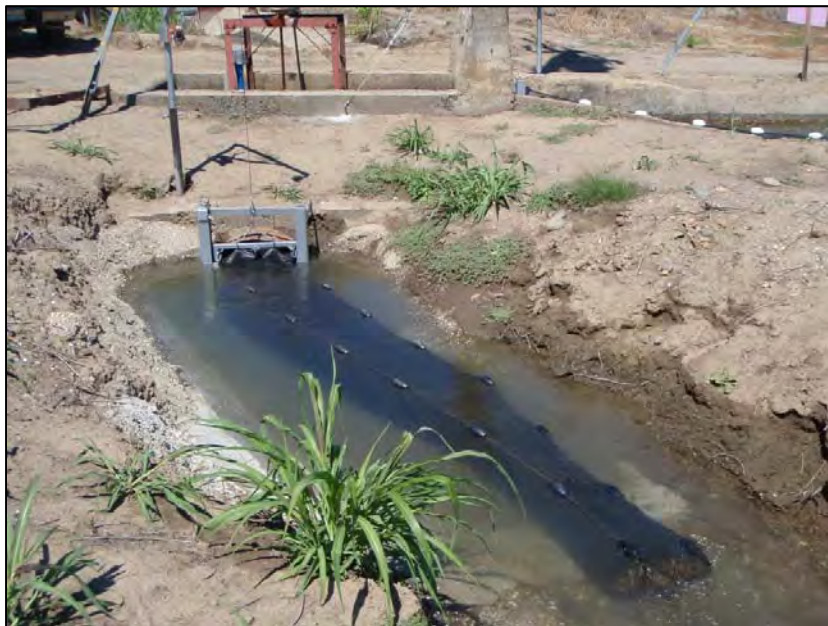
Figure 14. The fyke net and associated apparatus used to sample for fish entrainment in the Cranmore irregular-shaped concrete canal.
