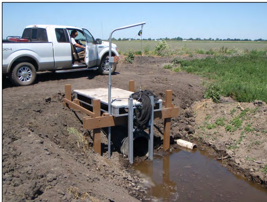
Figure 16. The fyke net, sampling platform, and associated apparatus used to sample for fish entrainment in the Sanchez west canal.
