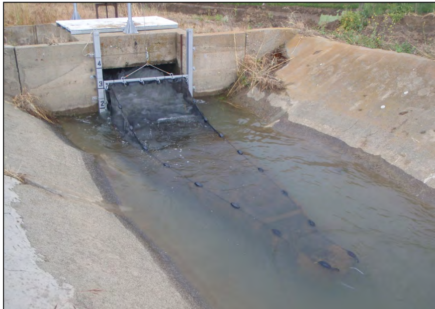
Figure 8. Fyke apparatus, fyke net, and sampling platform used to sample for fish entrainment in the Windswept canal.
