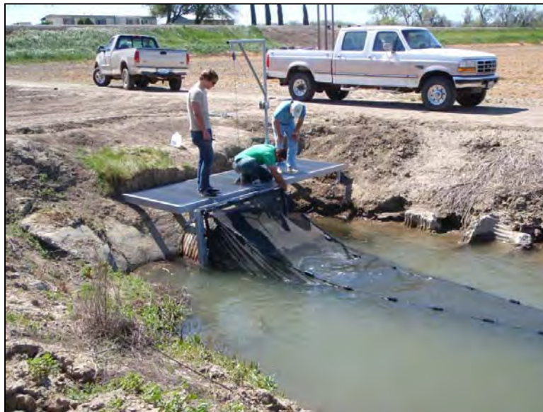
Figure 4. Fyke apparatus, fyke net, and sampling platform used to sample for fish entrainment in the State Ranch canal.
