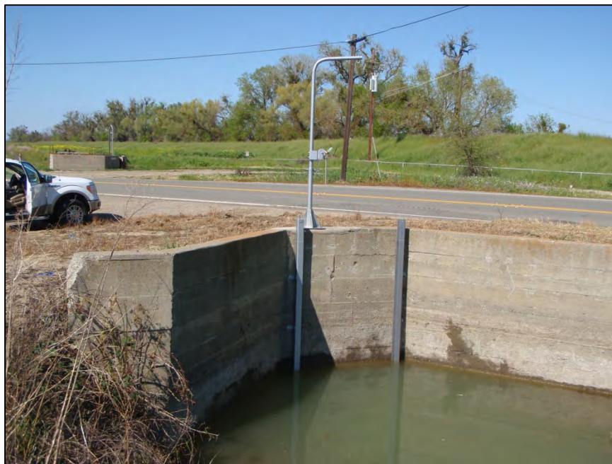
Figure 11. The fyke apparatus used to sample for fish entrainment in the Townsite south canal.
