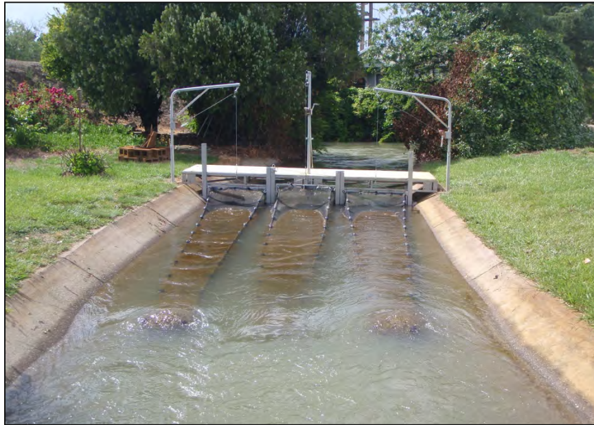
Figure 9. Three fyke nets, sampling platform, and associated apparatus used to sample for fish entrainment in the Portuguese Bend canal.
