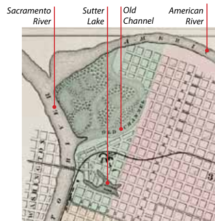
Figure 5.24. Old route of the American River. Before 1862, the American River's confluence with the Sacramento River was about a half mile downstream of its present confluence. It was rerouted to a more direct route to relieve flooding pressures on the city. (Ray 1873, courtesy of the David Rumsey Map Collection, Cartography Associates)
